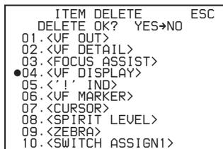
**3** To delete, turn the MENU SEL knob/ENTER button to move the arrow marker (⇒) to “YES,” and press the MENU SEL knob/ENTER button.
