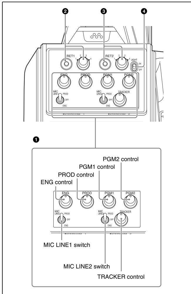
**1 INTERCOM1 and INTERCOM2 controls and switches**
