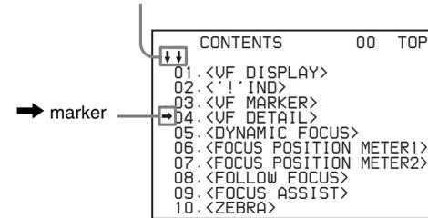
Turn the MENU SEL knob/ENTER button to align the arrow marker (➡) to the page to be set and press the MENU SEL knob/ENTER button.
