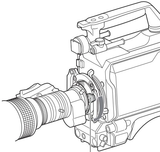
Lens fixing lever (B4)
