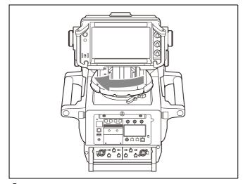
**4** Turn the slide position knob clockwise to **[]** FREE, and turn the slide-lock knob counterclockwise to release the lock of the slide position.
