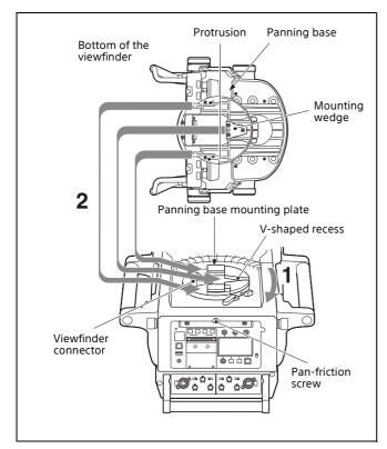
3 Press the base portion and insert the viewfinder fully into the panning base mounting plate. Pull the handle and check to ensure that the viewfinder
