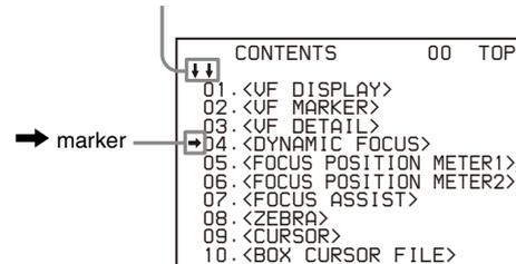
Turn the MENU SEL knob/ENTER button to move the arrow marker (➡) to the page to set, then press the MENU SEL knob/ENTER button.
