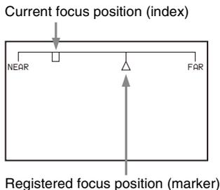
You can set the focus to the registered point easily by adjusting the focus until the index position overlaps the marker position (adjusted state). In the adjusted state, you can display a color frame and marker name on the viewfinder screen.
