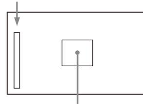
Area marker to display the detection area of the focus (its size and position can be adjusted.)
