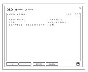
Click the  $\Delta$  (up) button and  $\forall$  (down) button at the bottom of the screen to switch between screens. Clicking the ENTER button applies/executes a setting. Clicking the CANCEL button cancels a setting.
