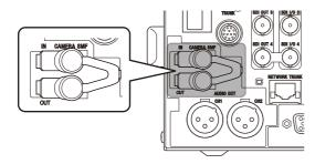
The CAMERA SMF IN connector inputs the video signal from the camera, audio (microphone) signal, HD-TRUNK signal, and NETWORK TRUNK signal.
