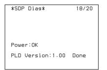
**Power:** Status of power supply to the SDP board **PLD Version:** SDP board PLD version
