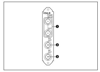
FRAME REF IN, OUT (frame reference input/output) connectors (BNC-type)
