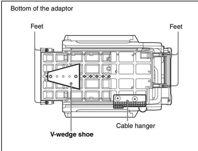
When attaching the V-wedge shoe, taking the total weight of the adaptor, camera, studio lens and viewfinder, and the size of the pan and tilt head of the tripod into consideration, choose a position such that the unit will be mounted stably on the tripod.
