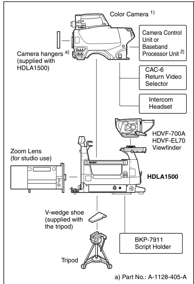
1) HDC4800, HDC4300, HDC3300/3300R, HDC2570, HDC2550, HDC2500, HDC2400, HDC1700, HDC1500/1500R, HDC1400/1400R, HSC-300, HSC300R/300RF
