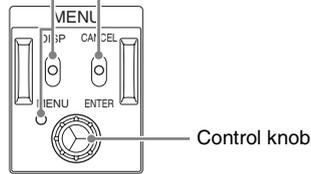
**DISP/MENU lever and indicator:** Used to display the status and menu. The indicator lights up when the menu is displayed.
