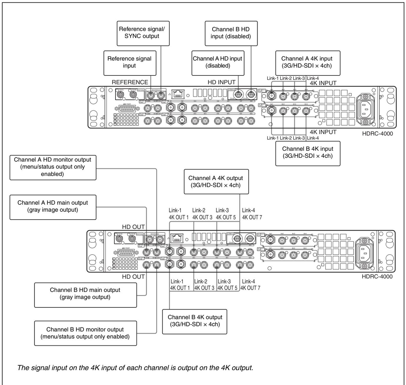
*The signal input on the 4K input of each channel is output on the 4K output.*
