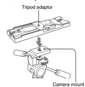
2 Mount the camcorder on the tripod adaptor.
