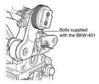
3 Adjust the front-to-back position so that the arm of the BKW-401 does not touch the handle when it is raised.
