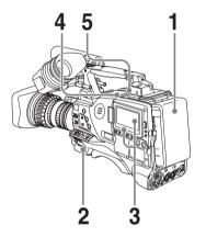
1 Attach a fully charged battery pack.
