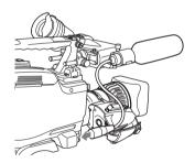
4 Secure the microphone cable with the cable clamps.
