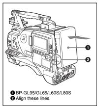
2 Slide the battery pack down until its "LOCK" arrow points at the matching line on the camcorder.
