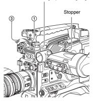
2 Couple the viewfinder connector to the VF connector.
