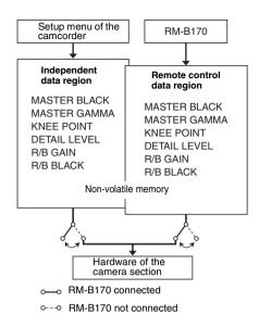
Thus, when a remote control unit is connected to the camcorder, the effective data region is switched to the "remote control data region" and the settings of the paint adjustment that were in effect the last time the remote control unit was used are recalled.
