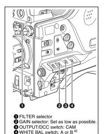
a)White balance setting values are stored in memory B only when the WHITE SWITCH <B> item is set to "MEM" on the WHITE SETTING page of the OPERATION menu.
