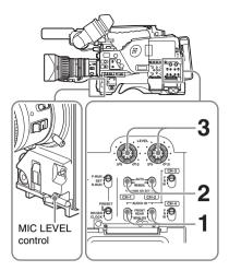
To adjust the signal input to the AUDIO IN CH1 or CH2 connector, set the AUDIO IN CH-1 or CH-2 switch to REAR.
