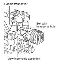
3 Attach the handle front cover with the bottom edge up.
