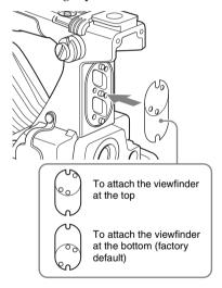
4 Attach the viewfinder slide assembly, reversing the steps of the removal procedure.
