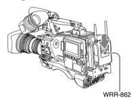
4 Connect the tuner power cord to the DC OUT connector of the camcorder, and the audio output cable to the AUDIO IN CH1 or CH2 connector.
