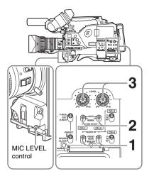
1 To adjust the signal input to the AUDIO IN CH1 or CH2 connector, set the AUDIO IN CH-1 or CH-2 switch to REAR.
