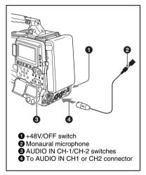
4 Switch the input level to match the sensitivity of the microphone used. Switch the input level by changing the REAR MIC REF setting on the AUDIO-1 page of the MAINTENANCE menu (factory default setting is -60 dB). For details, see page 173.
