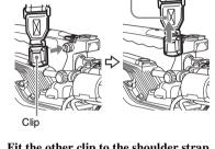
2 Fit the other clip to the shoulder strap fitting on the other side of the grip in the same way as in step 1.
