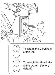
4 Attach the viewfinder slide assembly, reversing the steps of the removal procedure.
