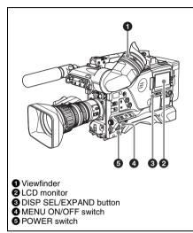
To use the MENU ON/OFF switch, open the cover of the menu operating section.
