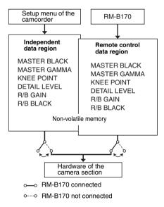
Thus, when a remote control unit is connected to the camcorder, the effective data region is switched to the "remote control data region" and the settings of the paint adjustment that were in effect the last time the remote control unit was used are recalled.
