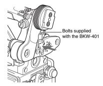
**3** Adjust the front-to-back position so that the arm of the BKW-401 does not touch the handle when it is raised.
