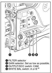
a)White balance setting values are stored in memory B only when the WHITE SWITCH <B> item is set to "MEM" on the WHITE SETTING page of the OPERATION menu.
