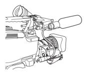
4 Secure the microphone cable with the cable clamps.
