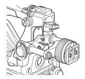
2 Using a 2.5 mm diameter hexagonal wrench, detach the viewfinder slide assembly and handle front cover.
