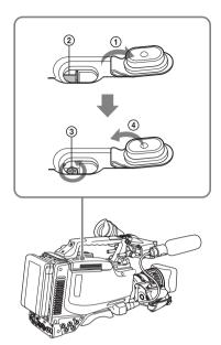
You need not return the screw to its original position after taking out the disc. Turning on the power makes the disc compartment mechanism operable again.
