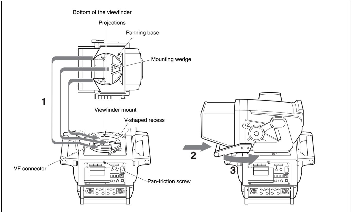
**1** Place the viewfinder on the viewfinder mount of the camera so that the mounting wedge on the bottom of the viewfinder enters the V-shaped recess on the viewfinder mount and that the projections on the bottom of the viewfinder are placed at the position shown in the figure above.
