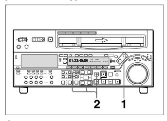
Press the RECORDER button or PLAYER button to select the VTR on which you wish to operate.
