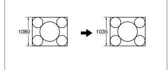
**1080** ⇒ **1035** (**CROP**): Convert the active scan lines from 1080 to 1035. Crop the top, bottom, left, and right, then stretch the image horizontally.
