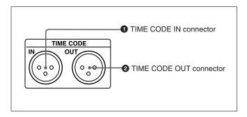
**1 TIME CODE IN connector (XLR 3-pin, female)** To record time code from an external device, input a time code signal from the time code output connector of the other device.
