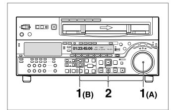
(A) Hold down the PLAY button, and turn the search dial in the desired direction to adjust the playback speed.
