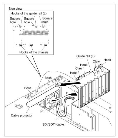
Remove the Cable Protector and Guide Rail (L)
