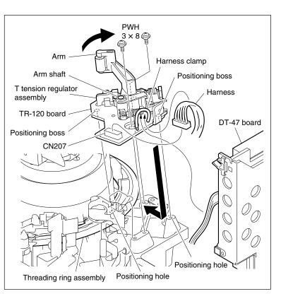
Attach the T Tension Regulator Assembly
