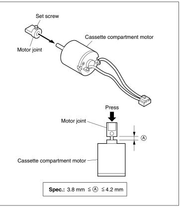
Attach the Motor Joint
