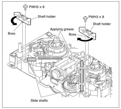
Reattach the Shaft Holder and Apply Grease
