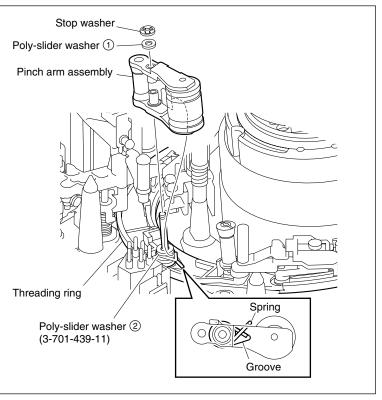
**Remove/Attach the Pinch Arm Assembly**
