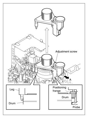
Figure 5. Removal of Head Tip Protrusion Measurement Gauge
