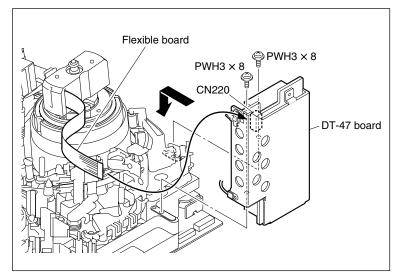
Reattach the DT-47 Board and Flexible Board
