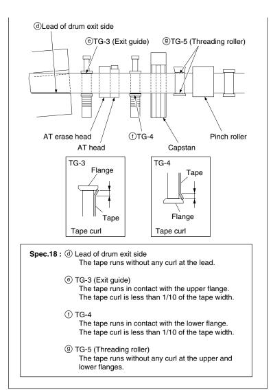
Tracking Adjustment at the Tape Exit Side
