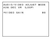
This menu is used to adjust the composite video input system.
