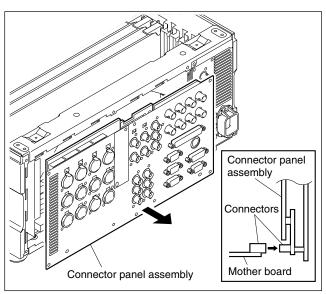
When reattaching, install in the reverse order of removal. **Note**
