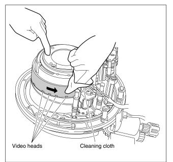
Figure 1. Cleaning of Drum
