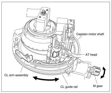
Confirm the CL Arm Assembly Operation
