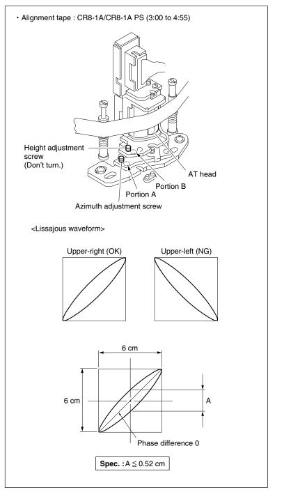
AT Head Azimuth Adjustment
