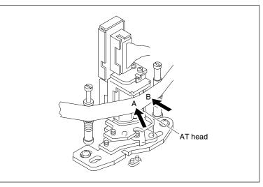
AT Head Head-to-tape Contact Check
