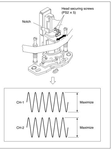
AT Head Head-to-tape Contact Adjustment
