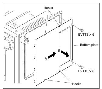
When reattaching, install in the reverse order of removal.
