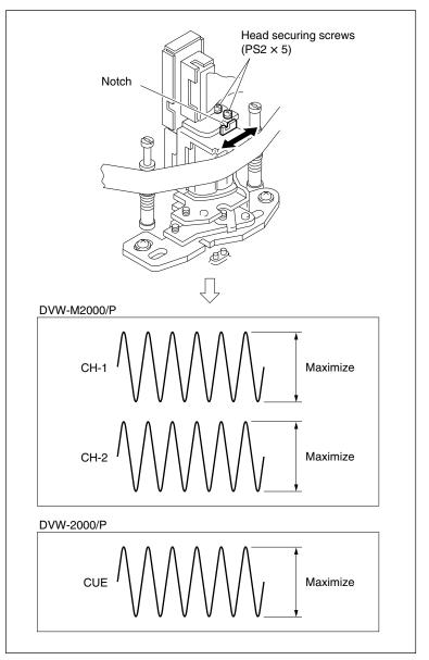
AT Head Head-to-tape Contact Adjustment
