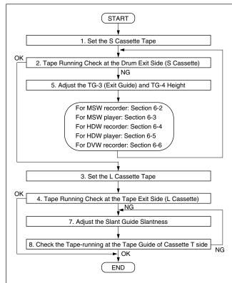
Flow Chart of Tape-running Check at Tape Exit Side
