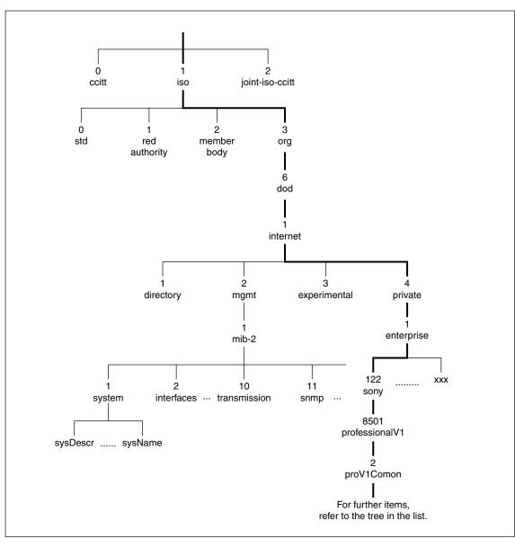
This section describes the MIB and trap description implemented in the e-VTR. The tree structure of the extended MIB is as follows:
