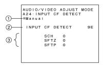
This menu is used to adjust the color frame detection timing of a composite video input signal. This is exclusive for the DVW/MSW recorder.
