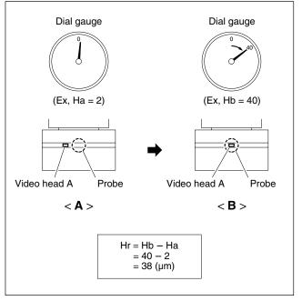
Figure 4. Example of Head Tip Protrusion Measurement
