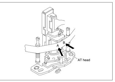
AT Head Head-to-tape Contact Check
