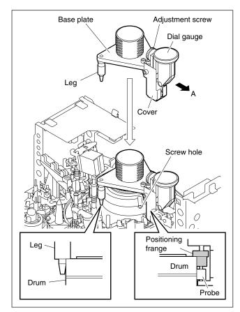
Figure 3. Setting of Head Tip Protrusion Measurement Gauge
