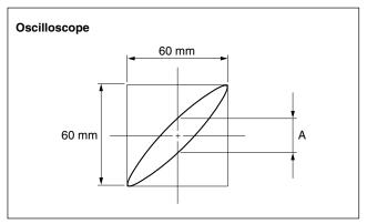
Figure 2. Lissajous Waveform of LAU PB Phase Adjustment
