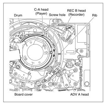
Figure 2. Setting of Drum Position
