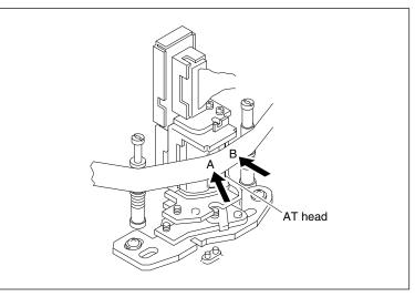
AT Head Head-to-tape Contact Check
