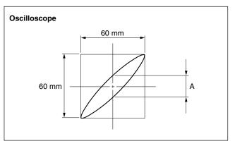
Figure 1. Lissajous Waveform of LAU PB Phase Adjustment
