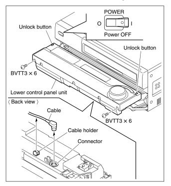
5. Lightly draw the lower control panel unit toward you, and then lift it upward.
