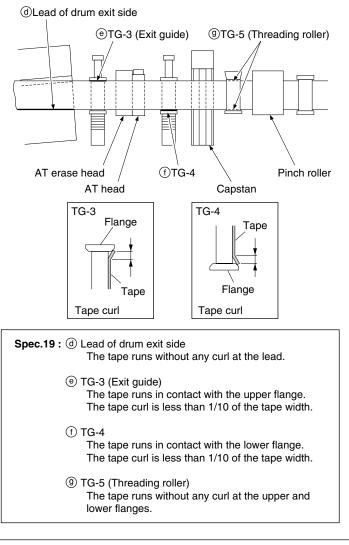
Tracking Adjustment at the Tape Exit Side
