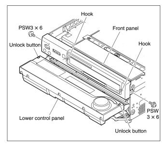
6. Release the three claws from the chassis, and remove the front panel in the arrow direction.
