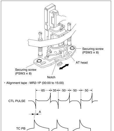
Spec. (for adjustment) :  $A = 0 \pm 0.6 \text{ ms}$
