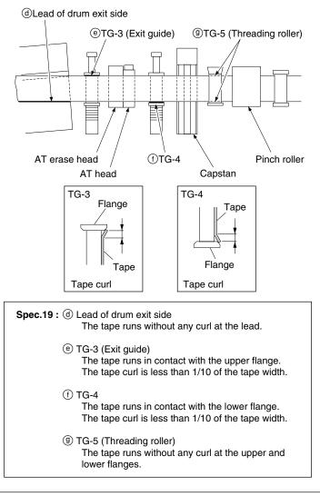
Tracking Adjustment at the Tape Exit Side
