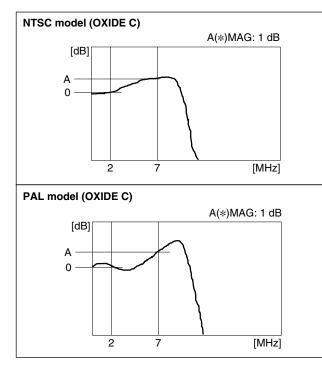
5. Adjust the delay time at 7 MHz using 2 MHz as the reference.
