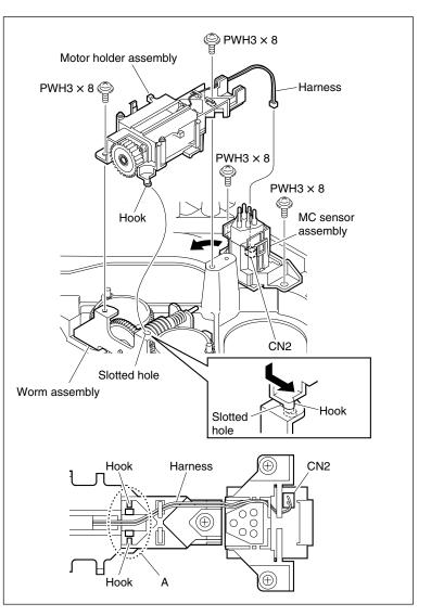
**Remove/Attach the Motor Holder Assembly**
