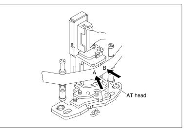
AT Head Head-to-tape Contact Check
