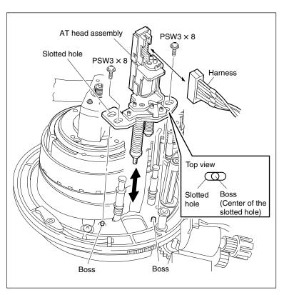
Remove/Attach the AT Head Assembly
