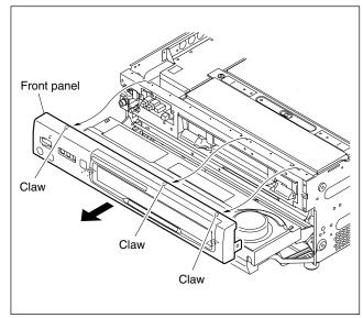
When reattaching, install in the reverse order of removal. **Note**
