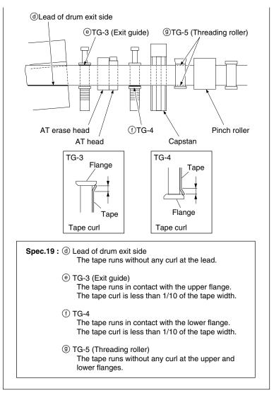
Tracking Adjustment at the Tape Exit Side
