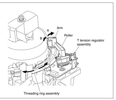
**T** Tension Regulator Assembly Operation
