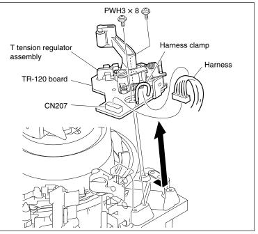
**Remove the T Tension Regulator Assembly**
