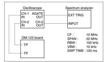
Connection and Setting of Spectrum Analyzer
