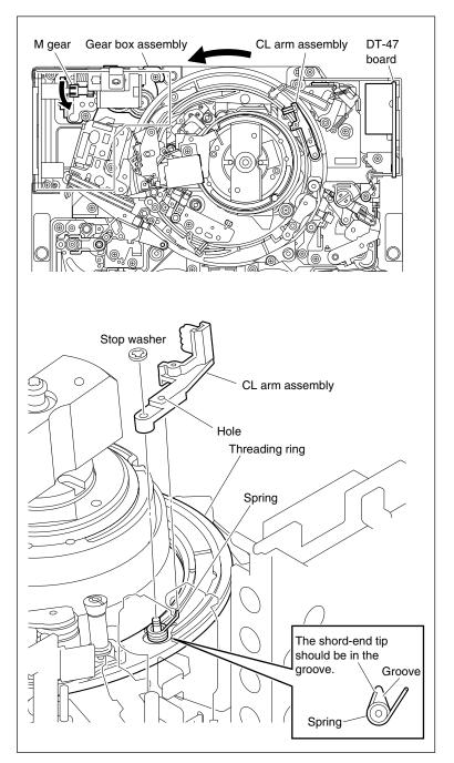
Remove/Attach the CL Arm Assembly
