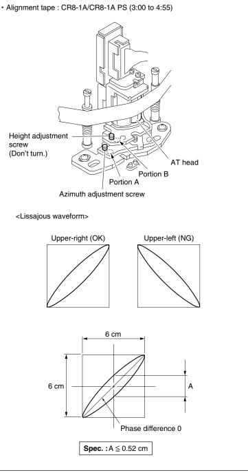
**AT Head Azimuth Adjustment**
