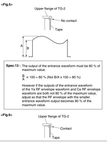
Analog Betacam Y/C Head Contact Adjustment
