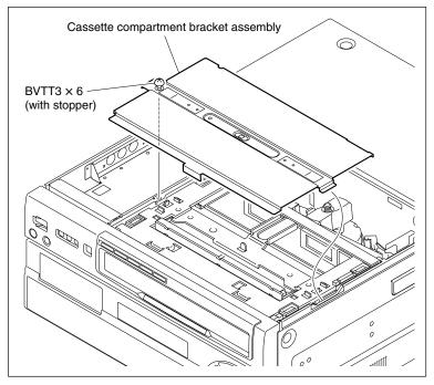
Remove the Cassette Compartment Bracket Assembly
