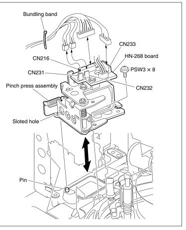
**Remove/Attach the Pinch Press Assembly**
