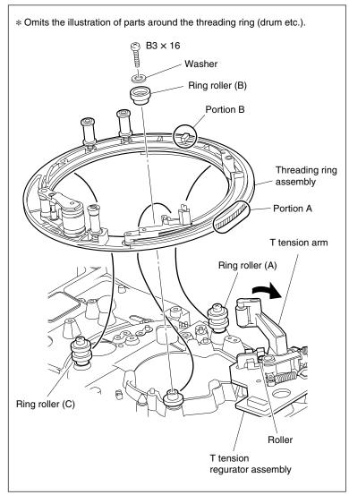
**Remove/Attach the Threading Ring Assembly**
