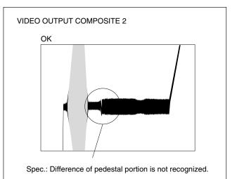
Figure 2. Pedestal Level Check
