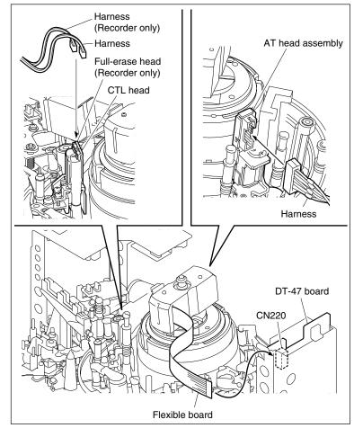
Connect the Flexible Board and the Harnesses
