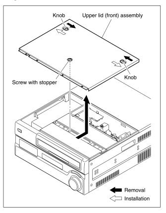
When reattaching, install in the reverse order of removal.
