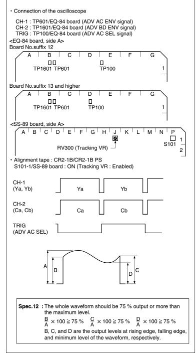
Analog Betacam Y/C Head Contact Check
