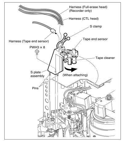
Remove/Attach the S Plate Assembly (New Type)
