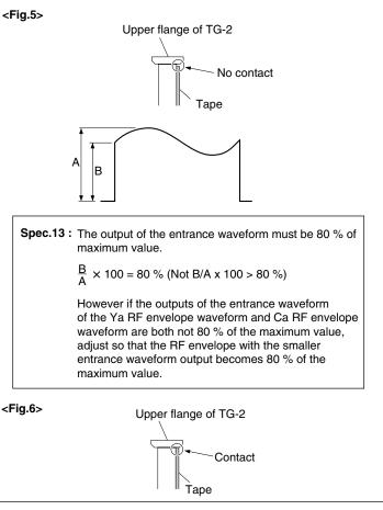
Analog Betacam Y/C Head Contact Adjustment
