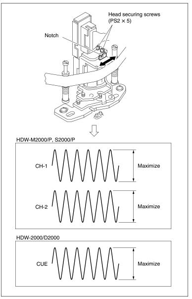
AT Head Head-to-tape Contact Adjustment
