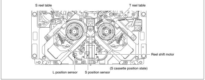
Locations of S and L Position Sensors and Reel Shift Motor
