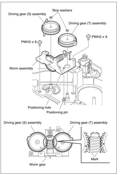
**Remove/Attach the Drive Gear Assemblies**
