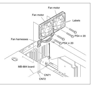
Remove/Attach the Fan Motor
