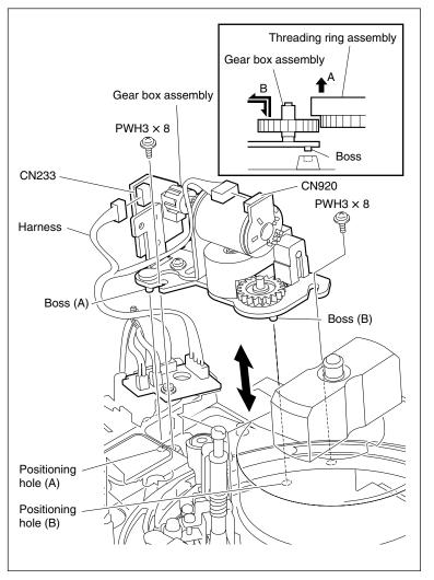
Remove/Attach the Gear Box Assembly
