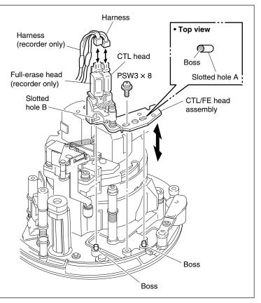
Remove/Attach the CTL/FE Head Assembly
