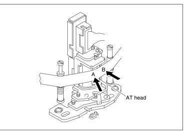
AT Head Head-to-tape Contact Check
