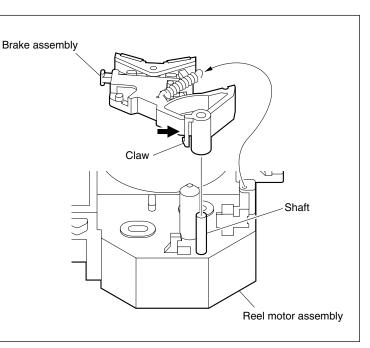
**Remove/Attach the Brake Lining**
