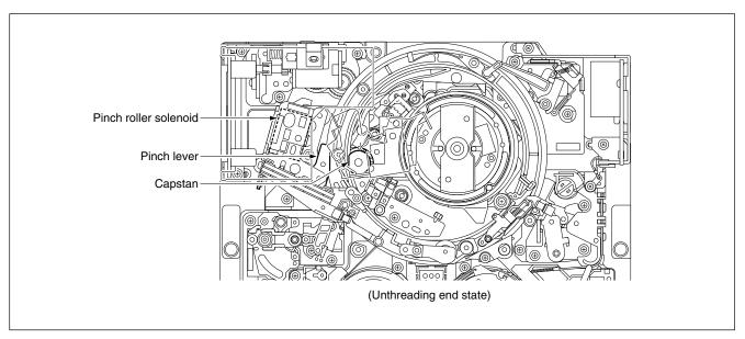
Locations of Pinch Roller Solenoid and Pinch Lever
