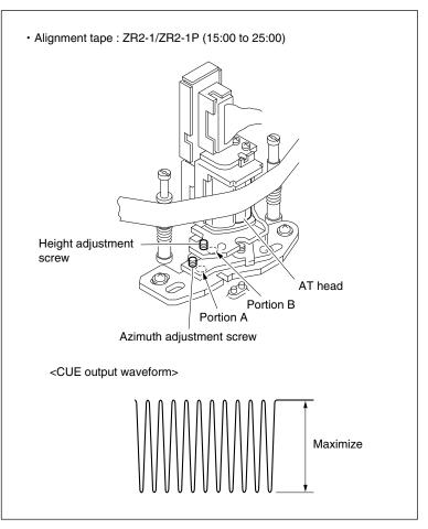
AT Head Azimuth Adjustment
