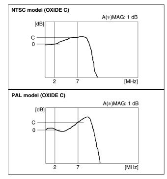
Set the data of "MAIN OXIDE-C-B" in A34 : COS EQ VR (OXIDE-C) to the identical data value as "MAIN OXIDE-C-A".
