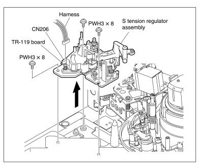
**Remove the S Tension Regulator Assembly**
