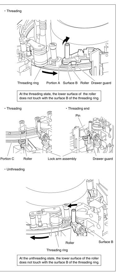
**Confirm the T Drawer Assembly Operation**
