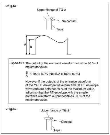
Analog Betacam Y/C Head Contact Adjustment
