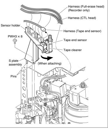
Remove/Attach the S Plate Assembly (Former Type)
