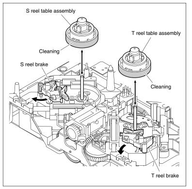
**Remove/Attach the Reel Table Assembly**
