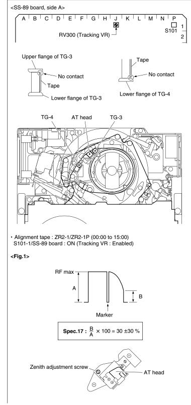
(8) Turn the height adjustment nut of TG-3 clockwise so that the tape is in contact with the upper flange and the RF envelope waveform becomes flat. (Fig. 2)Simultaneously, ensure that the tape does not in contact with the lower flange of TG-4.
