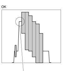
Spec.: The white level of the signal after looping overlaps on the white level of the 1st signal.
