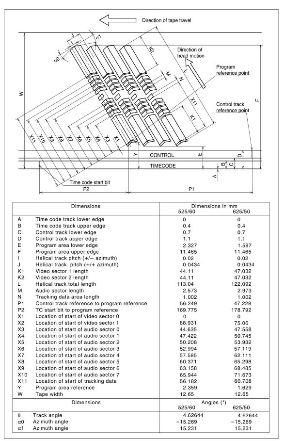
Fig. 10-2-2. Detail of MPEG IMX Format Tape Pattern
