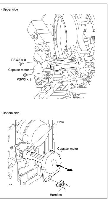
**Remove/Attach the Capstan Motor**
