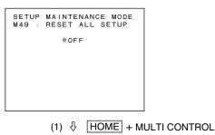
SETUP MAINTENANCE MODE M49 : RESET ALL SETUP \*ON Push SET Button ----- Caution -----All the System Setup data will be changed to Factory default.
