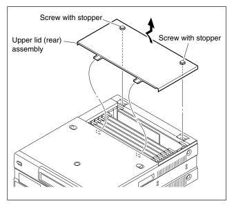
When reattaching, install in the reverse order of removal.
