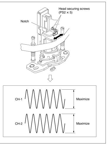
AT Head Head-to-tape Contact Adjustment
