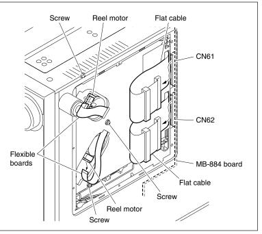
**Disconnect the Flat Cables and Flexible Boards**
