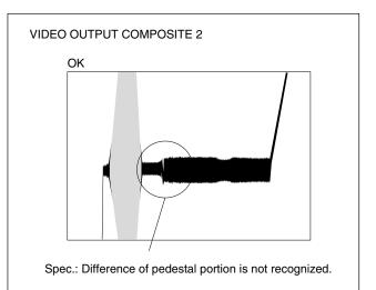
Figure 2. Pedestal Level Check
