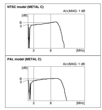
9. Set the data of "MAIN METAL-C-B" in A32 : COS EQ VR (METAL-C) to the identical data value as "MAIN METAL-C-A".
