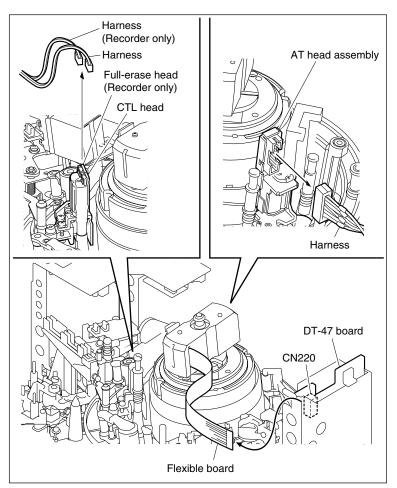
Disconnect the Flexible Board and the Harnesses
