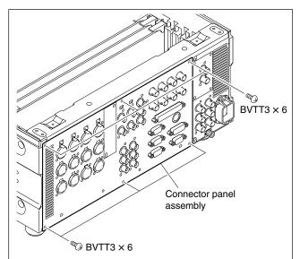
4. Push out the connector panel assembly from inside the unit in the arrow direction, and disconnect the connector connected to the mother board.
