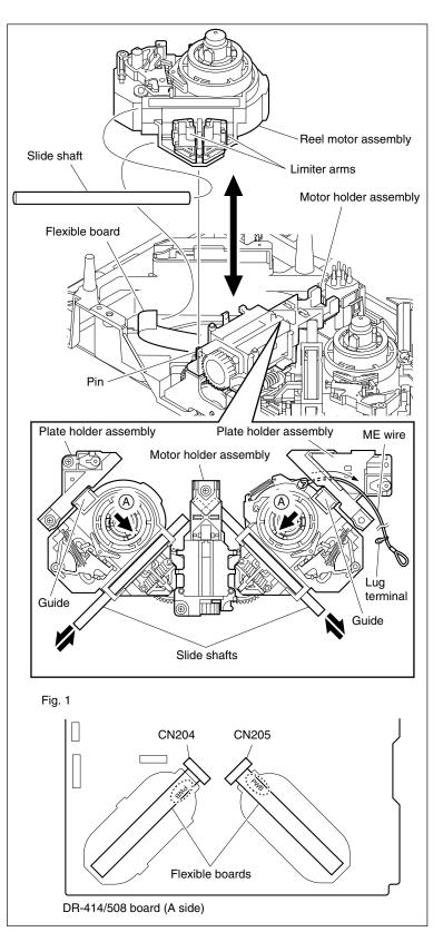
Remove/Attach the Reel Motor Assembly
