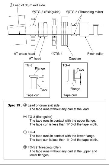
Tracking Adjustment at the Tape Exit Side
