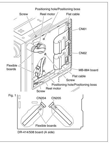
**Connect the Flat Cables and Flexible Boards**
