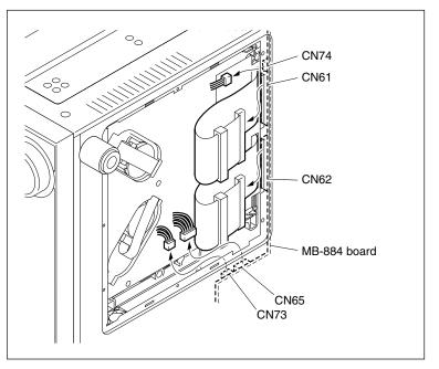
Disconnect the Flat Cables and Harnesses (1)
