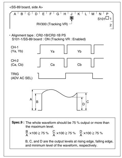
Analog Betacam Y/C Head Contact Check
