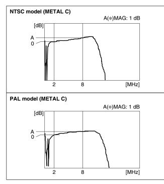
6. Adjust the group delay time in 3 MHz through 9 MHz. Adj. points: ⊘RV301/DM-123(L-3) and ⊘RV302/DM-123(L-2)
