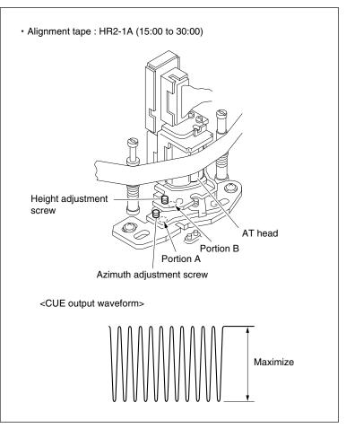
AT Head Azimuth Adjustment
