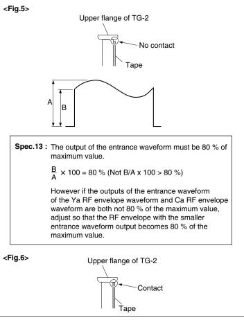
Analog Betacam Y/C Head Contact Adjustment
