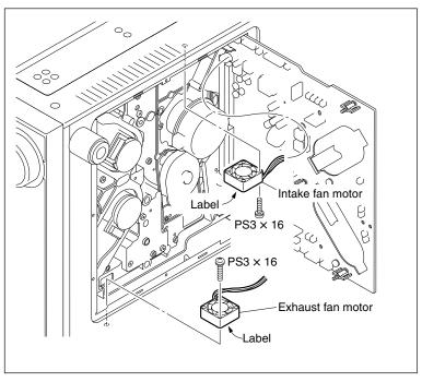
Remove/Attach the Fan Motor
