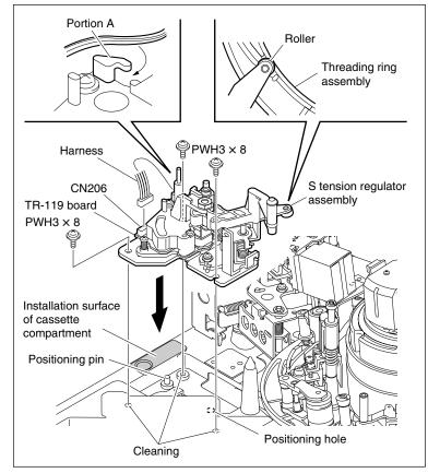
Attach the S Tension Regulator Assembly
