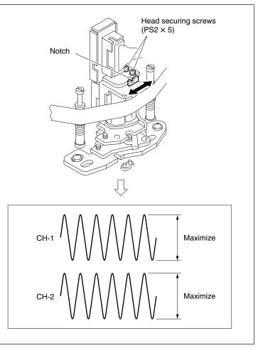
AT Head Head-to-tape Contact Adjustment
