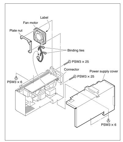
**Remove the Power Supply Unit**
