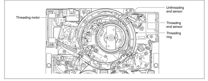
Locations of Threading End and Unthreading End Sensors
