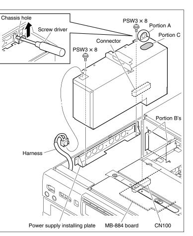
Remove/Attach the Power Supply Unit
