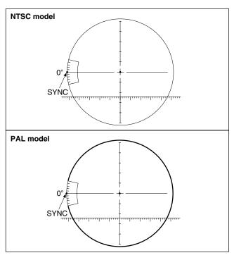
Composite waveform/vector monitor (SCH mode)
