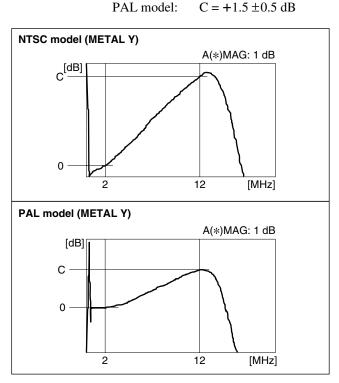
11. Set the data of "MAIN METAL-Y-B" in A31 : COS EQ VR (METAL-Y) to the identical data value as "MAIN METAL-Y-A".
