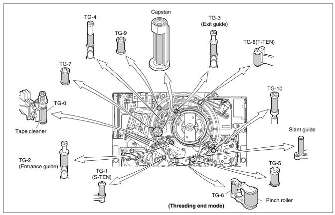
**Tape-running System and Tape Cleaner Cleaning**
