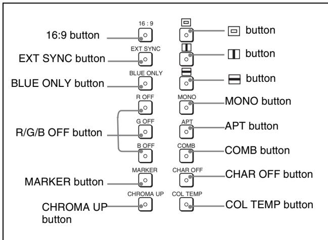
**☐ (Under scan) button:** When this button is pushed in (ON), the picture is under scanned by 3%, and four ends of the raster is displayed on the screen.
