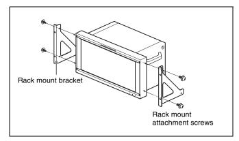
**3** Screw the rack mount brackets to the rack to mount the unit.
