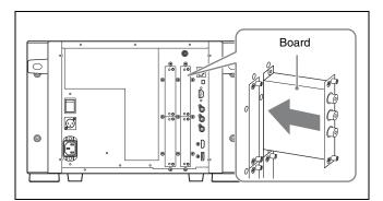
**3** Push the adaptor in until it is firmly fit into the connector inside the monitor, then tighten the two screws to secure the adaptor.
