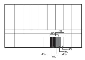
4 Adjust so that the luminance of the 100% white signal of the color-bar is set to the desired value with the CONTRAST knob.
