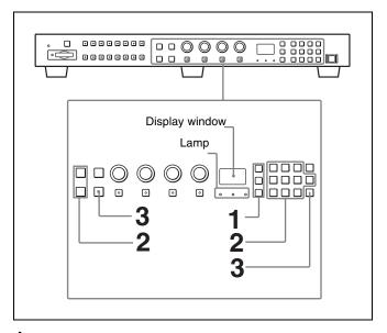
**1** Press the corresponding button to select the connection mode.
