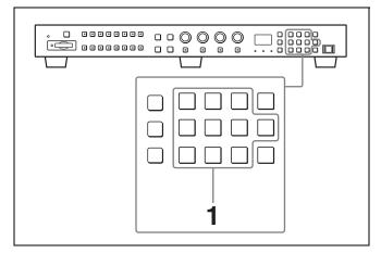
1 Select the channel (CH1 to CH30) to be assigned by pressing the numeric button of the controller.
