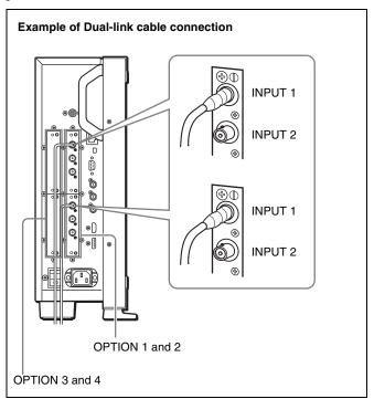
When the BKM-250TG is used, install the Link A signal to INPUT 1, and the Link B signal to INPUT 2.
