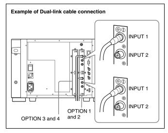
When the BKM-250TG is used, install the Link A signal to INPUT 1, and the Link B signal to INPUT 2.
