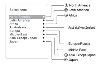
Press the UP or DOWN button of the controller to select the area where you intend to use the monitor and press the ENTER (Ent) button.
