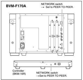
**2** Set the different IP address to each monitor and the controller.
