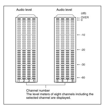
Audio Level Meter and ALM Hold Reset are assigned to the function buttons of the controller in the Function Key menu (page 83) of the Controller menu.
