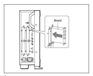
**3** Push the adaptor in until it is firmly fit into the connector inside the monitor, then tighten the two screws to secure the adaptor.
