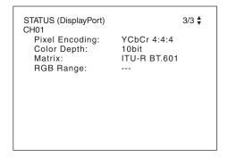
**Pixel Encoding:** RGB 4:4:4 / YCbCr 4:4:4 / YCbCr 4:2:2 **Color Depth:** 8bit / 10bit / 12bit (HDMI signal), or 6bit/8bit/10bit/12bit (DisplayPort signal) **Matrix**<sup>1)</sup>: ITU-R BT.601 / ITU-R BT.709 **RGB Range**<sup>2)</sup>: Limit / Full
