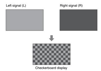
The left (L) and right (R) signals are displayed in a checkerboard pattern on the same screen for comparing the brightness or colors of the L and R signals.
