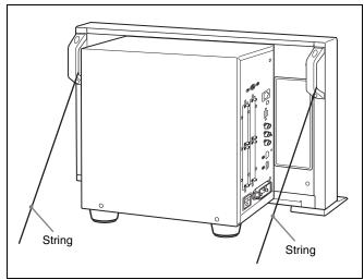
**2** Secure the ends of the string to the floor or wall.
