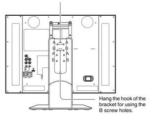
**5** Secure the arm with four screws.
