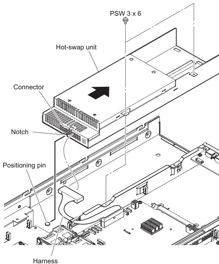
4. Install the removed parts by reversing the steps of removal.
