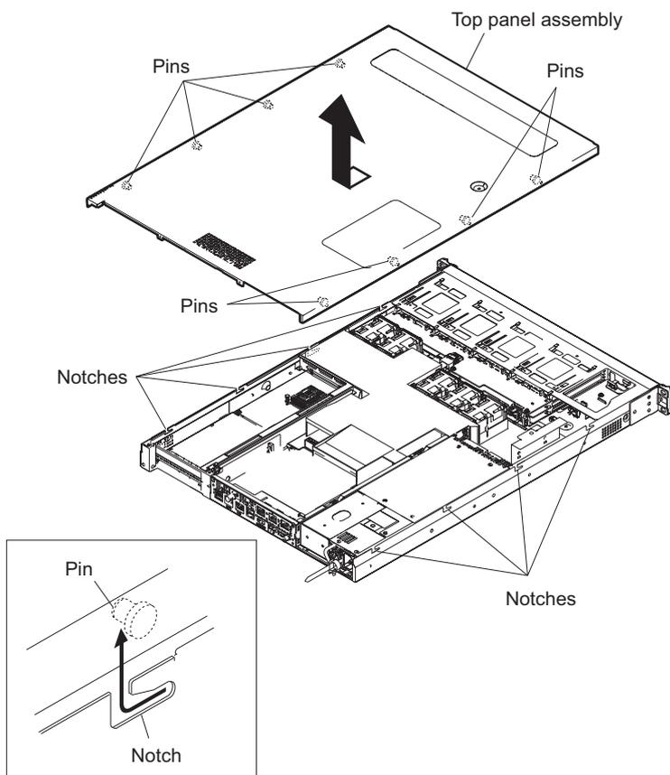
3. Install the removed parts by reversing the steps of removal.
