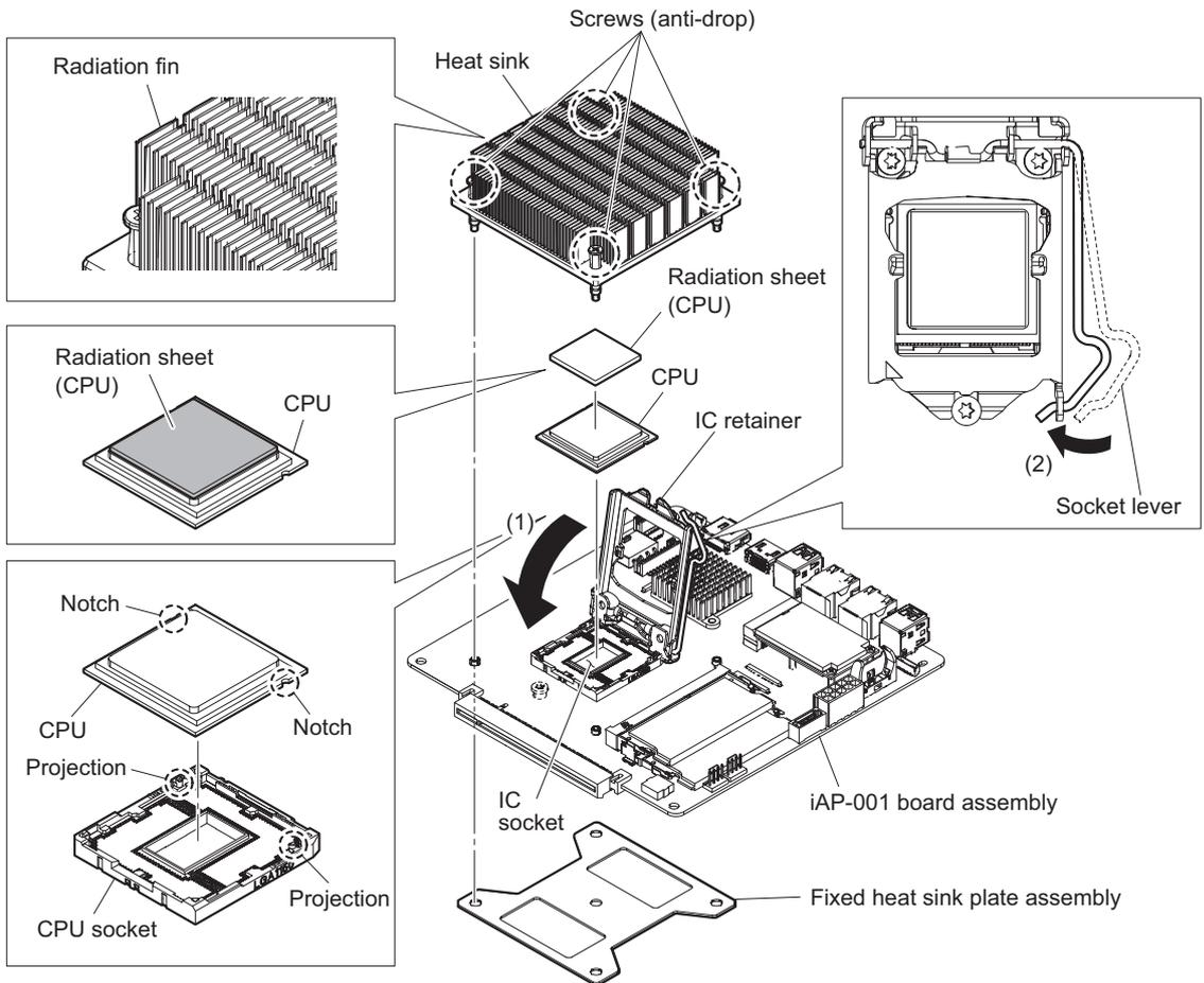
11. Assemble this unit by reversing the steps of "Preparation".
