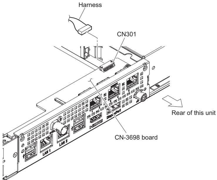
2. Remove the screw (B2.6 x 5) and the screw (PSW3 x 6) to detach the CN-3698 board in the direction of the arrow.
