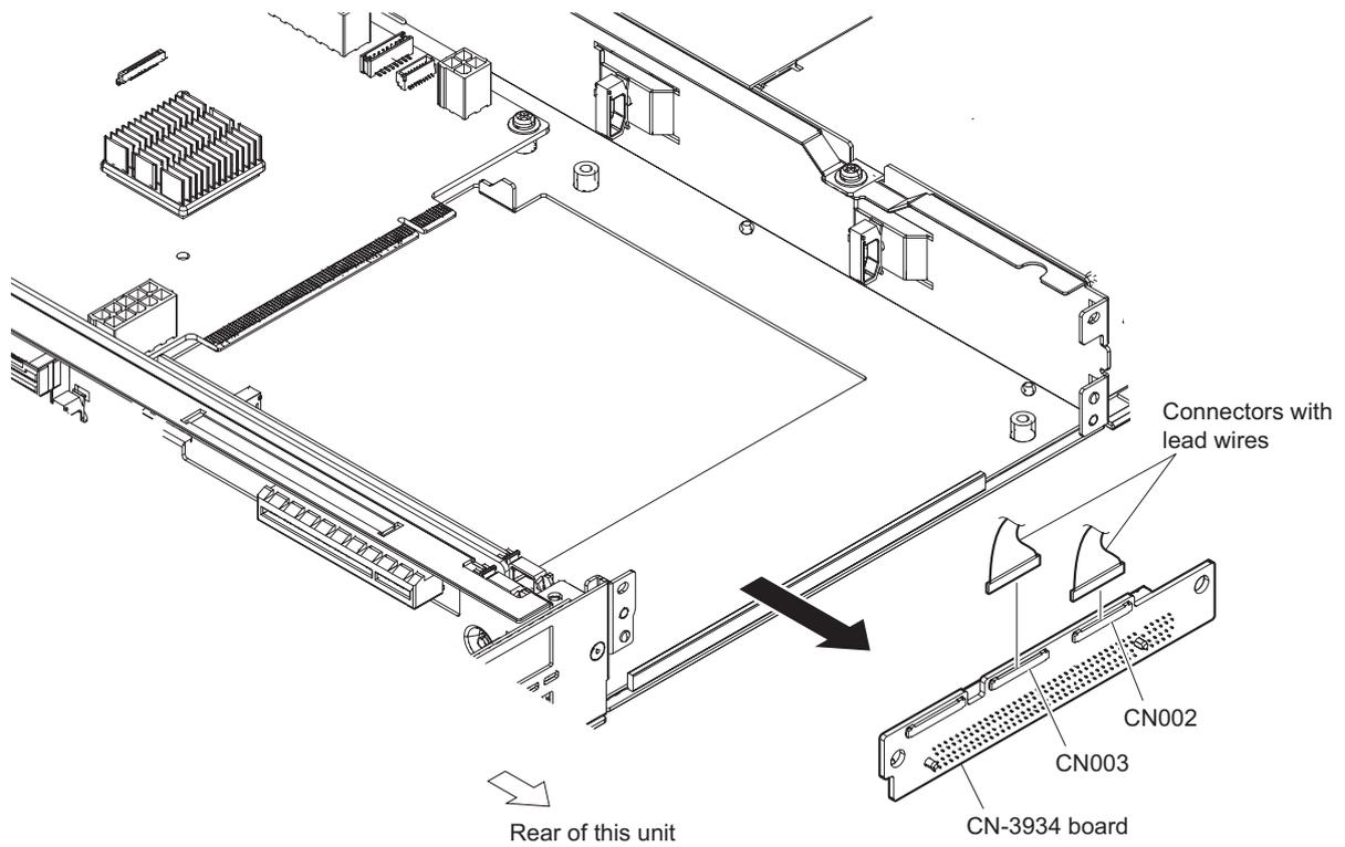
3. Install the removed parts by reversing the steps of removal.
