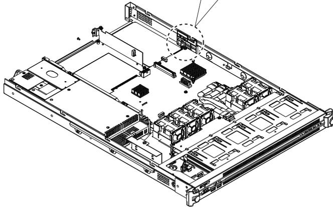
4. Remove the three screws and release the four hooks, then remove the MB-1204 board in the direction of the arrow.
