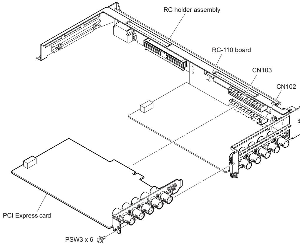
5. Remove the screw, then remove the lower PCI Express card from the connector (CN102) on the RC-110 board in the same way as the upper slot.
