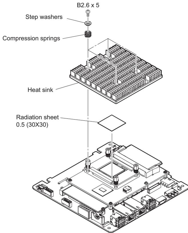
3. Remove the five screws, and then remove the iAP-005 CPU board from the connectors on the IF-1330 board.
