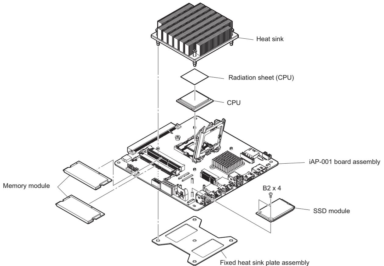
9. Install the removed parts by reversing the steps of removal.
