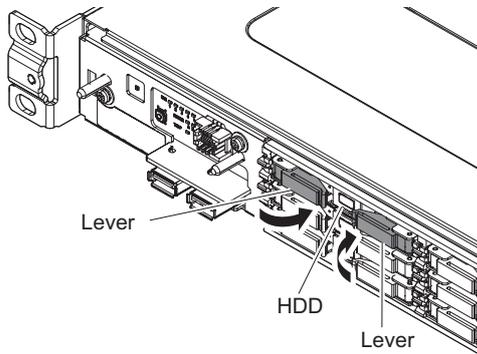
5. Remove a piece of number label from the ST-No sheet and attach it to the front of the HDD assembly.
