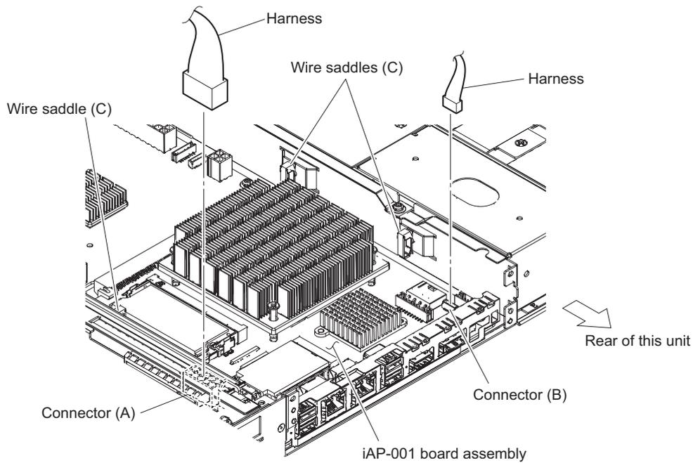
3. Remove the four screws and detach the iAP-001 board assembly in the direction of the arrow.
