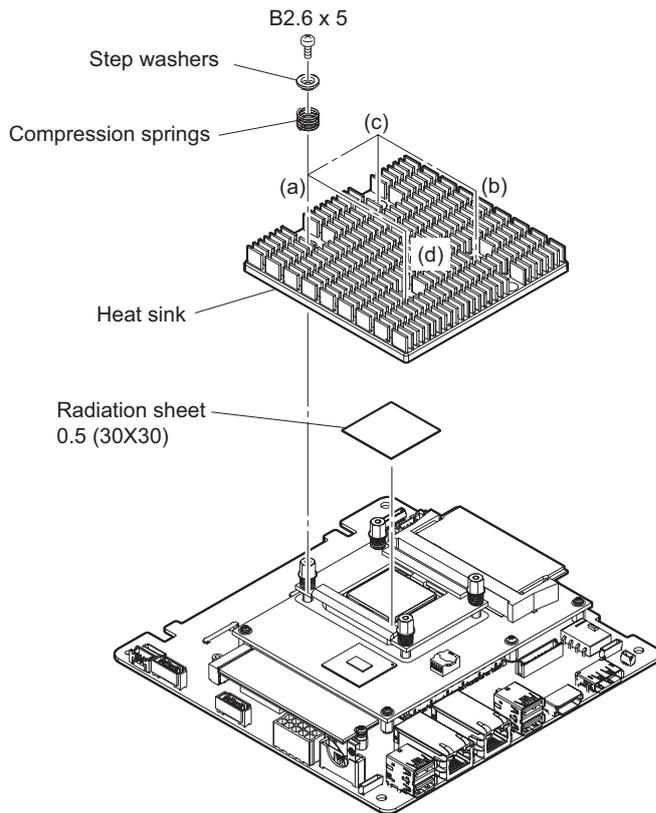
17. Assemble the unit by reversing the steps of "Preparation".
