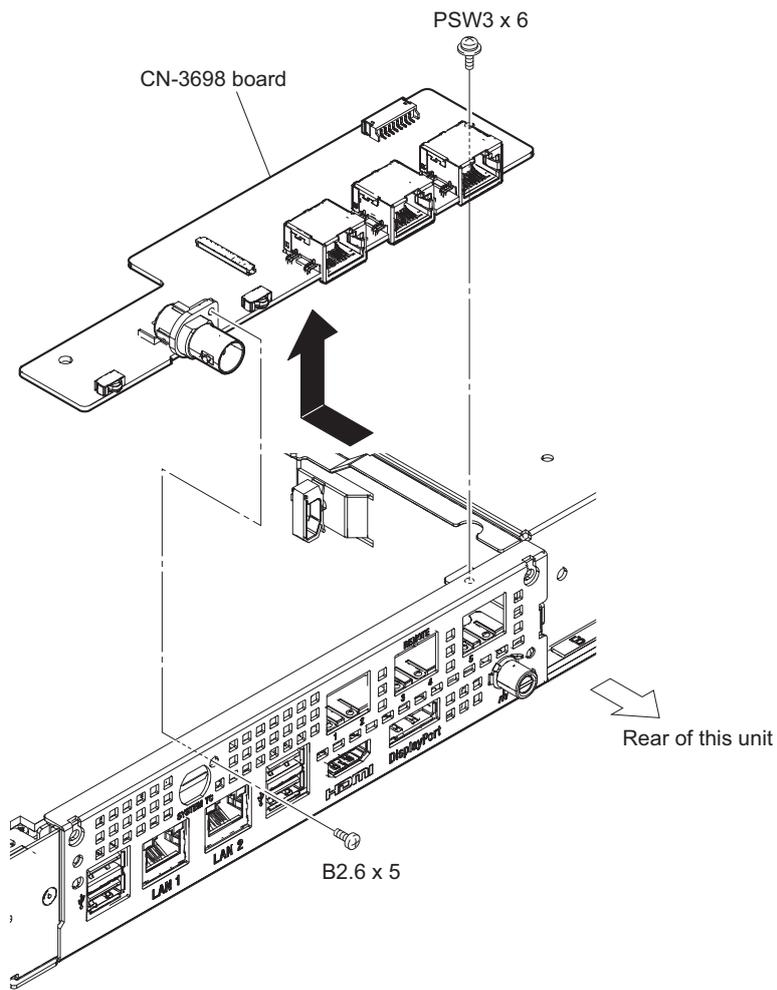
3. Install the removed parts by reversing the steps of removal.
