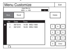
8 Use the numeric keypad or the leftmost adjustment knob to select the file number, and press Enter.
