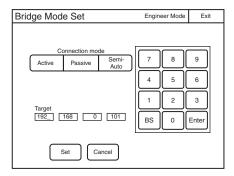
② Press a button to set the sub mode (Connection mode) of BRIDGE mode.
