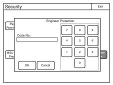
3 Use the numeric keypad to enter any security code (1 to 8 digits), and then press OK.
