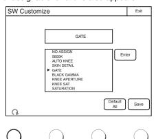
7 Turn the adjustment knob on the far left to select the function to assign to the button.
