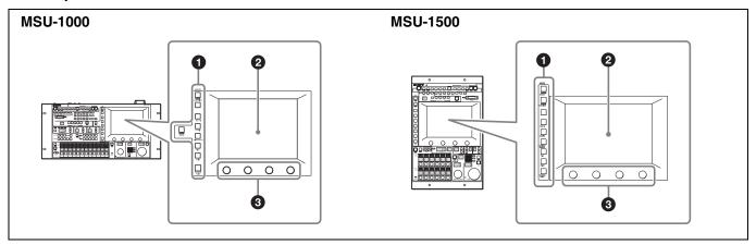
Menu operation is performed on the LCD. Operation is performed by touching the buttons and tabs that are displayed on the LCD. Use the adjustment knobs to change numbers and select items.
