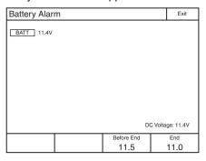
Use this screen for setting the battery alarm. Set the items as required.
