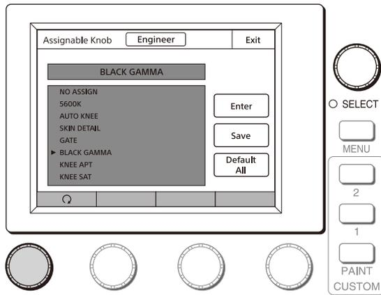
**3 Turn the adjustment knob on the far left to select the function to assign to the assignable adjustment knob.**
