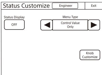
This status display screen ON/OFF button, the status screen type select button, and the menu customize button of the adjustment knobs (according to display type) are displayed.
