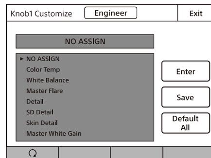
**5** Turn the adjustment knob on the far left to select the function assigned to the adjustment knob.
