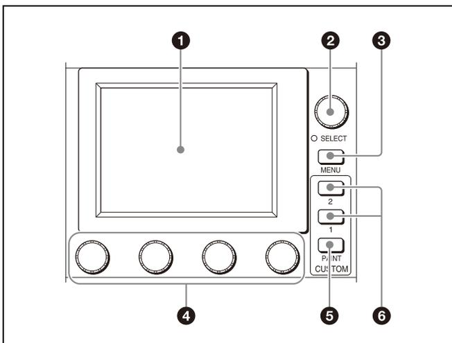
The menu operation block is used to configure the camera and CCU using the LCD and touch panel. Select a menu item using the SELECT knob, and change the adjustment value of the selected item using the four adjustment knobs.
