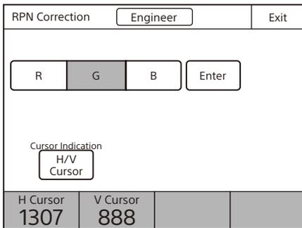
When you press **RPN** in the Maintenance menu, a cross-shaped cursor appears on the PIX monitor connected to the CCU. Perform the following steps while viewing the PIX monitor.
