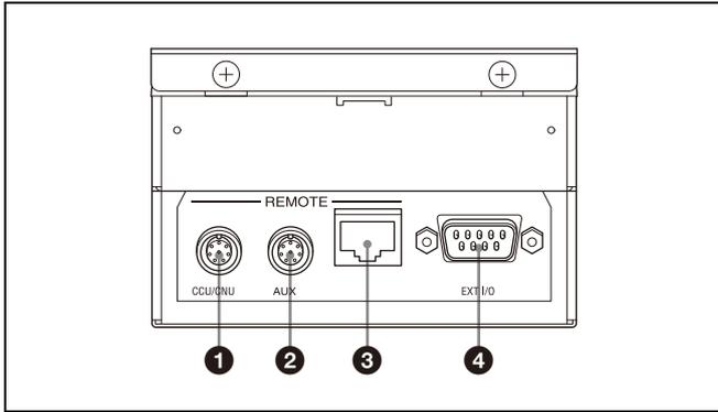
**1 CCU/CNU REMOTE (CCU/CNU remote) connector (8-pin multi-connector, female)**
