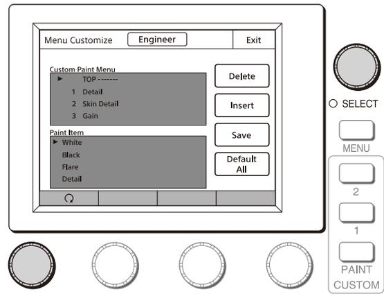
This screen contains two lists, one at the top and the other at the bottom. The top list displays the custom paint menu items. The bottom list displays the paint menu items that can be added to the custom paint menu. You can edit the custom paint menu by selecting paint menu items in the bottom list and adding them to the top list.
