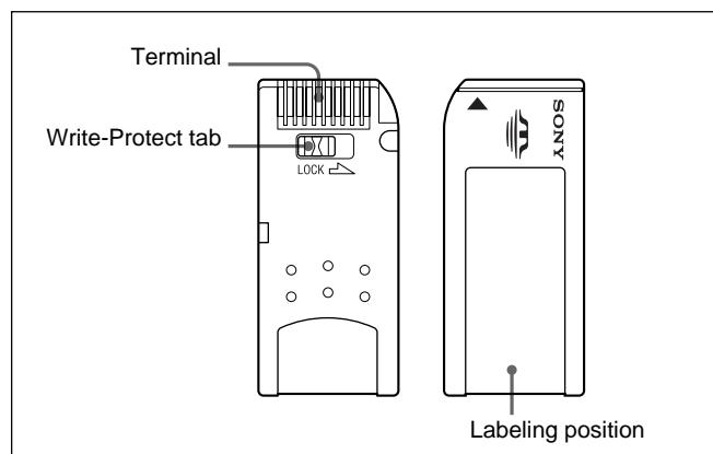
You cannot record or erase data when the write-protect tab on the **Memory Stick** is set to LOCK.
