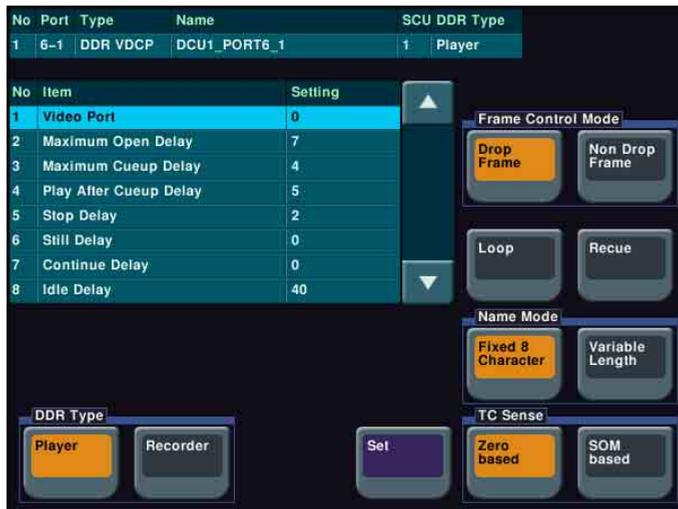
When “Simple VDCP” is selected as the protocol, the Simple VDCP Setting menu appears.
