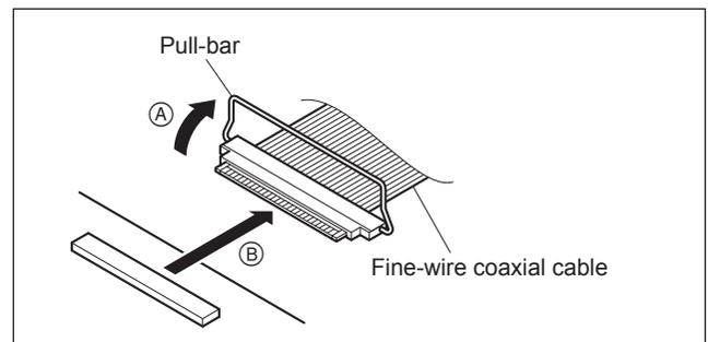
1. Raise the pull-bar in the direction of arrow (A) to unlock it, and then disconnect the fine-wire coaxial cable in the direction of arrow (B).
