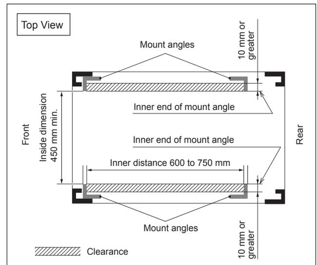
Be sure to mount this unit into a rack accurately following the procedure and notes mentioned below.
