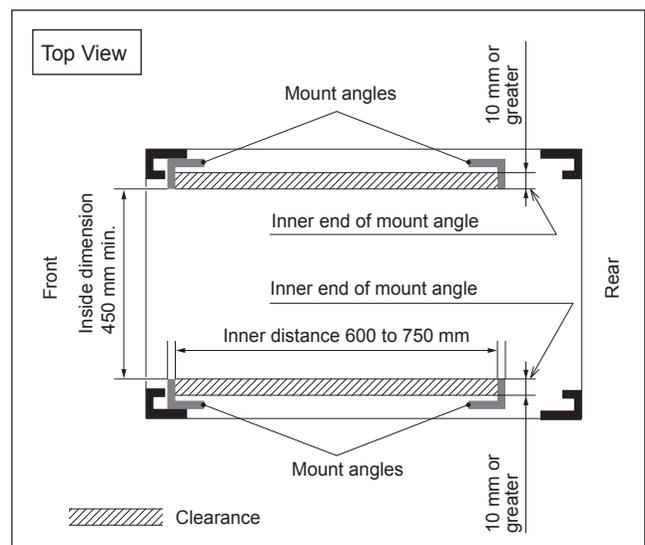
Be sure to mount this unit into a rack accurately following the procedure and notes mentioned below.
