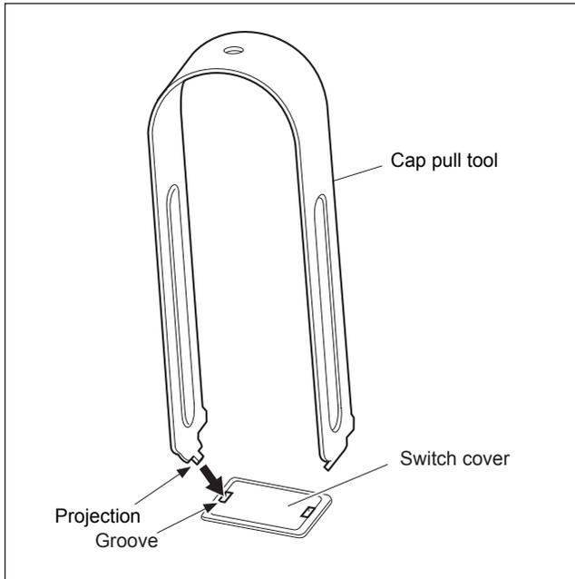
7. Hold and pull the cap pull tool in the direction of arrow to detach the switch cover.
