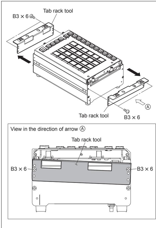
3. Set the tab rack tool at the position shown in the figure, and then install it with four screws.
