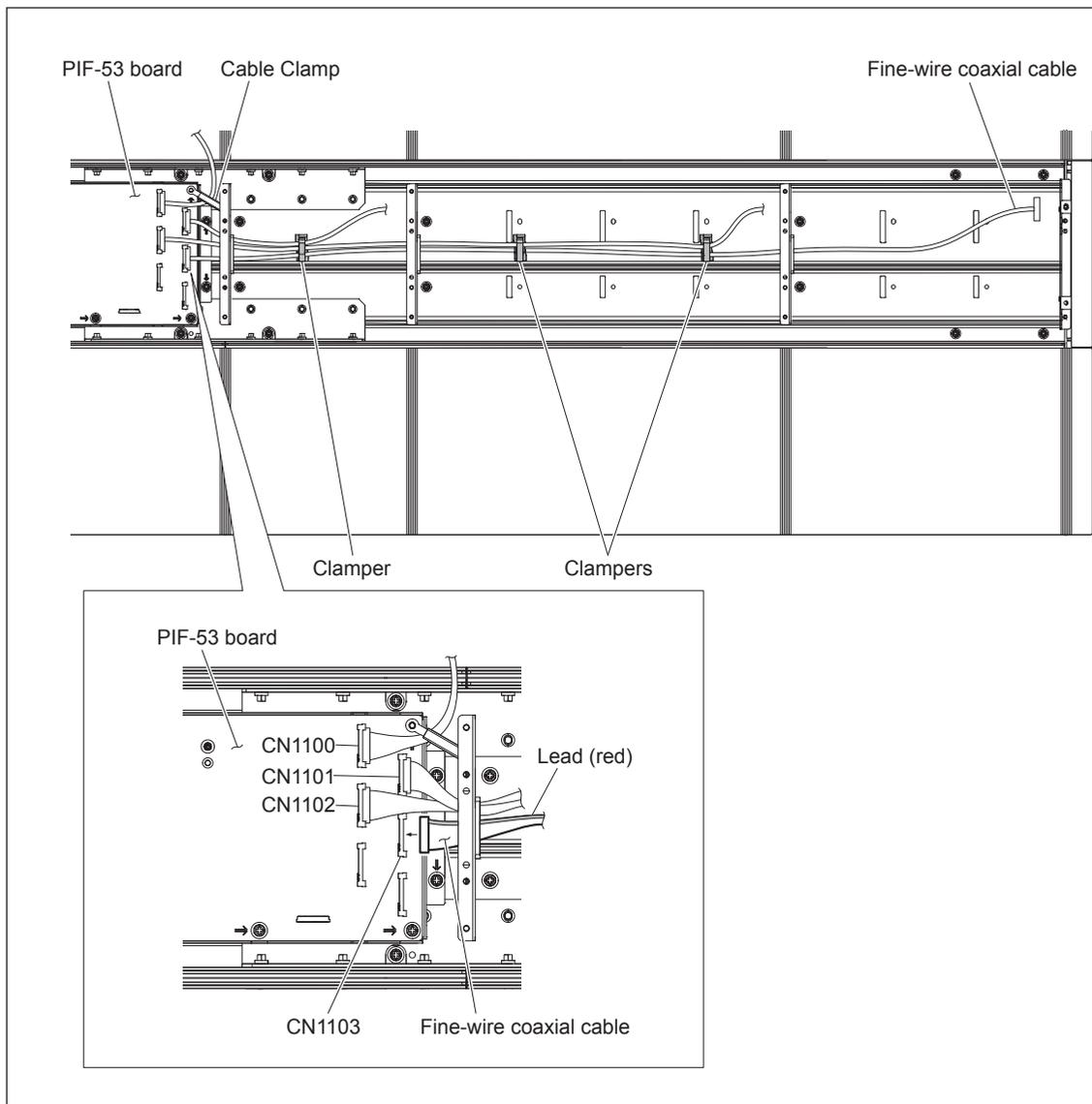
6. Connect the fine-wire coaxial cable to the connector on the operation module to be installed newly.
