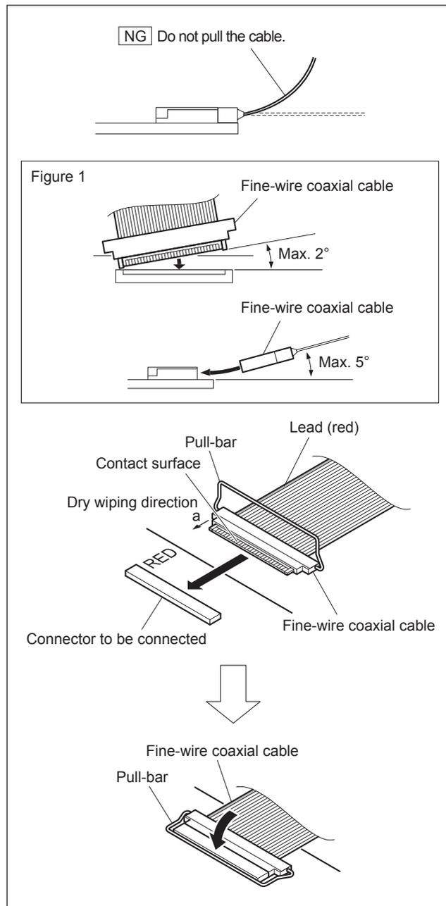
1. Wipe the contact surface with a dry wiping cloth in the direction of arrow (a).
