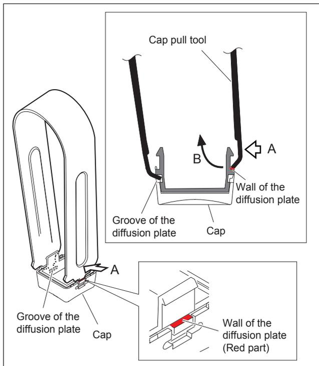
4. Remove the current label and install the new label to the cap.
