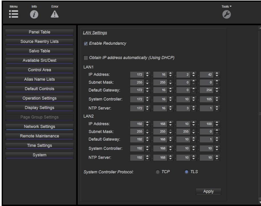
2. Clear the “Obtain IP address automatically (Using DHCP)” checkbox, and then make LAN1 network settings.
