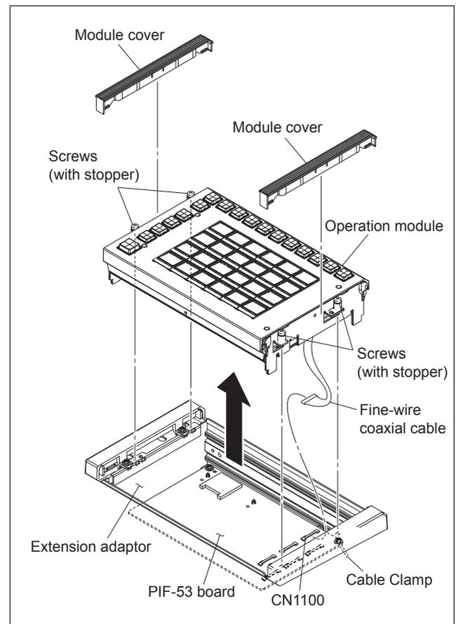
5. Connect the fine-wire coaxial cable to the connector (CN1100) on the PIF-53 board, and clamp the cable with a cable clamp.
