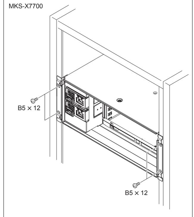
9. Attach the front panel to the equipment.
