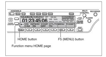
With the function menu HOME page showing in the menu display, press the F5 (MENU) button. The currently selected setup menu item is displayed in the menu display, with the menu item number flashing.
