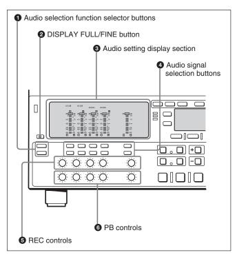
In the audio control section, you can select and display input and output signals for audio channels.
