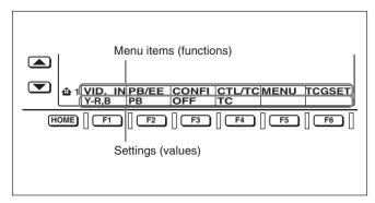
In the figure above, Y-R,B (analog component signals) is selected as the setting for VID.IN, the menu item for button F1. This manual refers to this as "F1 (VID.IN) in function menu HOME page is set to Y-R,B."
