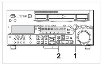
1 Press the RECORDER button or PLAYER button to select the VTR on which you wish to operate.
