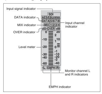
**Input signal indicator:** Indicates the currently selected input signal ('SDI', 'AES/EBU', 'ANA' for analog) for the corresponding audio input channel.
