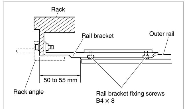
16. To fix the two outer rails to the rack, fully tighten the eight loosely fitted hexagon socket head cap screws in step 12 using the L-shaped hexagon wrench.
