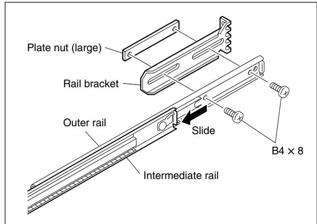
11. Slide the ball retainer in the direction of the arrow, and then loosely attach the front rail bracket to the outer rail with a plate nut (large) and the two screws.
