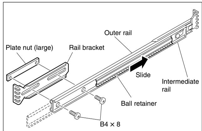
• **Attaching the outer rails**
