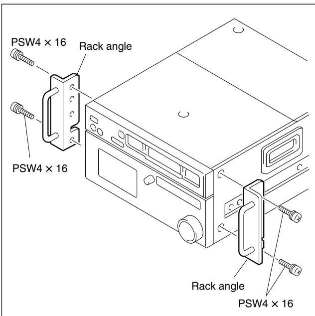
• **Loosely attaching the rail brackets**
