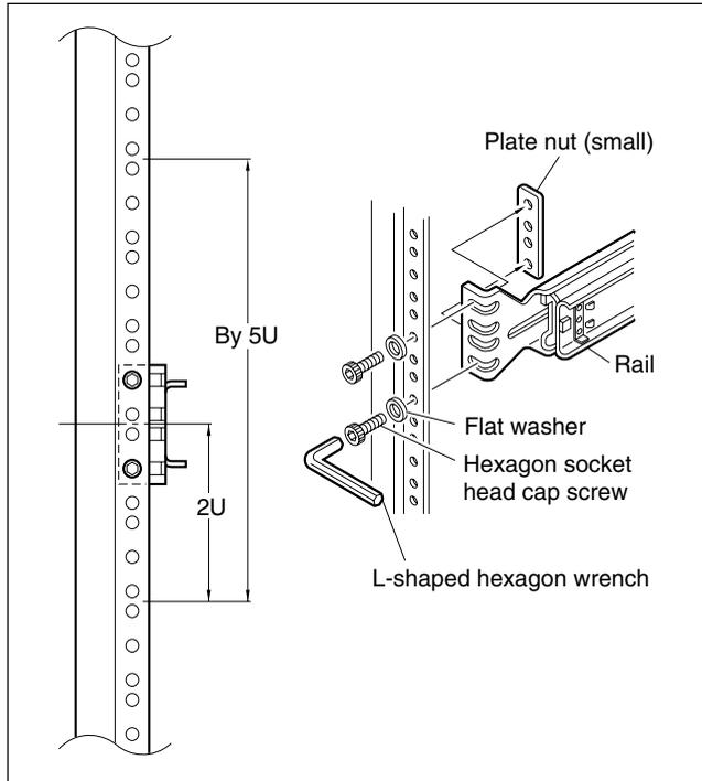
13. Check that the two intermediate rails attached to the rack are parallel.
