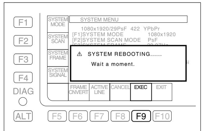
(3) Check that the system is restarted, and turn OFF the POWER switch and turn ON again.
