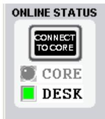
Only when there is a second network connection from the Virtual Vista computer to the second port of the SCore Live's bridge card - the Virtual Vista can be connected to the core.
