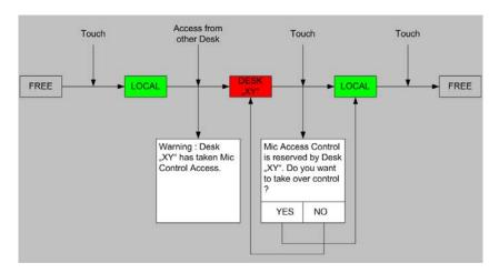
With the Vista desk, this dialog is handled in the channels Vistonics<sup>TM</sup> view in order to be able to link a number of channels and do the take-over handling for all of these channels at the same time (with a 'gang').
