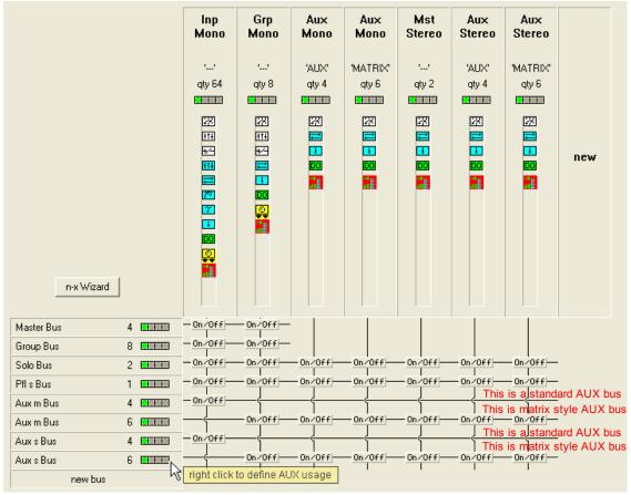
In order to avoid confusion about which master is a "true" auxiliary master and which one is a matrix output, we recommend you rename the user label of the "matrix style" master channels to.
