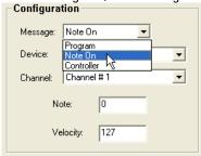
MIDI Out: Program change, note change, controller and sysex commands may be fired off by this event. A TEST button allows sending out this parameter during system setup without recalling the cue.
