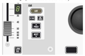
They can be used to control various functions of the cue list and allow certain functions to be switched using a hardware key, while it remains possible to use the trackball and operate these functions on the graphic controller screen:
