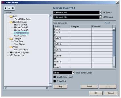
**Note:** In Cubase/Nuendo, the controller #4 must be mapped to Ethernet MIDI port 1, controller #3 to Ethernet MIDI port 2, etc., as shown in the screenshots above, in order to get the correct order of DAW channels 1 through 32 on the Vista console.
