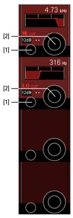
HI CUT/LO CUT [1] Slope setting for the high- and low-cut filters, selectable from 12, 18, and 24 dB/octave (toggles 12, 18, 24, 12, ...).
