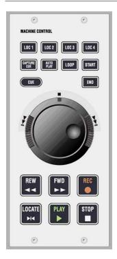
An optional machine control panel can be fitted into the Vista 8 control bay. This gives control over one external machine using Sony P2 ("Sony 9-pin") protocol. Please contact Studer Service & Support for installation instructions.
