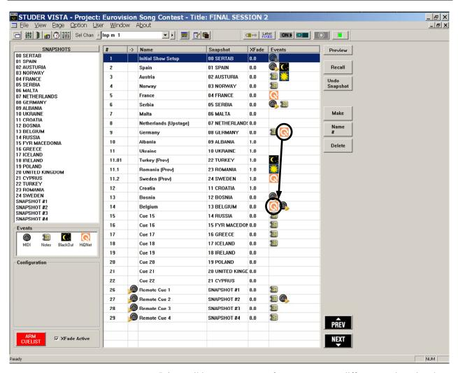
It is possible to move events from one cue to a different one by using dragand-drop. Also, snapshots may be moved between cues using drag-anddrop. In this way, snapshots can be replaced or exchanged within cues.
