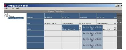
When finished, click the Save IO Sharing button at the right-hand edge of the Configuration Tool GUI.
