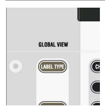
If the second layer option is activated, Vista 8 may display the label and real time metering of both layers at the same time. In order to activate this label view, press LABEL TYPE several times until the label display area on the Vistonics<sup>®</sup> screen shows the labels of both layers. This label of the second layer appears only if there is a channel assigned to that strip on both layers. Use the Strip Setup dialog on the graphic controller screen to do this.
