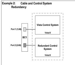
In the examples above, the (single) bridge card must be installed in slot 10 of the SCoreLive frame; the maximum number of DSP cards is 9.
