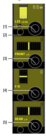
**LFE LEVEL [1]** This is a simple level trim for the LFE leg of the surround signal. The default level is 0 dB. Maximum boost/cut is +10 dB/-90 dB.
