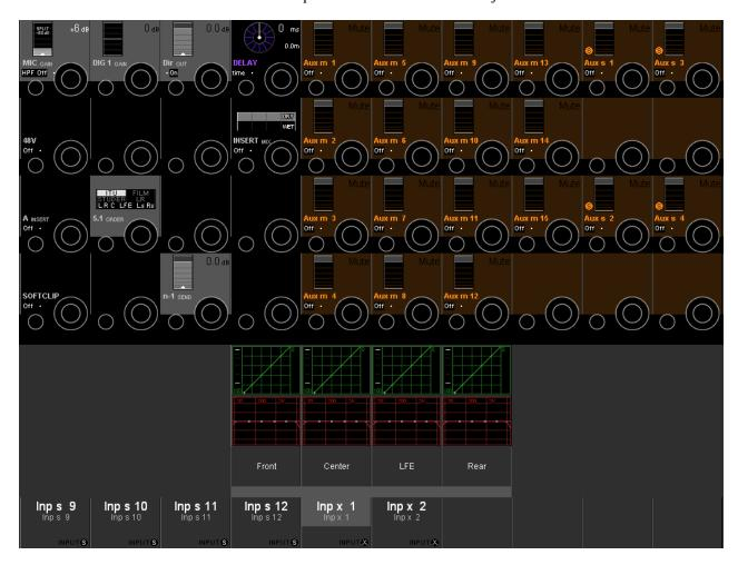
As can be seen above, there is an additional selection possibility in the touch area that allows modifying the EQ and dynamics parameters for the Front, Center, LFE and Rear signals individually.
