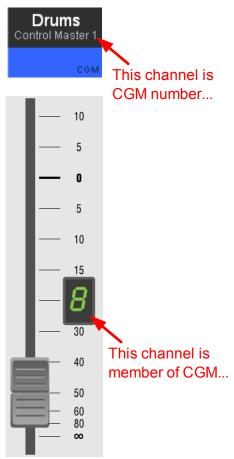
D950: On the D950 it is not possible to see, to which CGM a CGM may belong. A small light next to the fader shows the presence of another hierarchical level.
