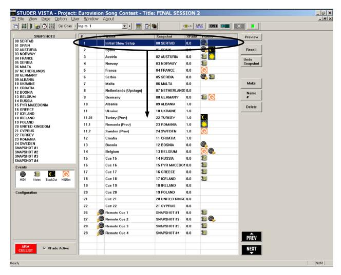
Automatic numbering example: When inserting a cue between the cues 11 and 12, this cue will automatically be numbered 11.1. If another cue is inserted between 11 and 11.1, this new cue will be numbered 11.01. Please note that he system doesn't allow further cues to be inserted between 11 and 11.01 without manually modifying the number 11.01 first.
