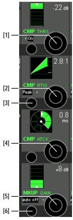
CMP THRS [1] The compressor threshold level can be adjusted in 1 dB steps from  $0 \ dB_{FS}$  to  $-96 \ dB_{FS}$ .
