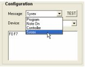
**MIDI Out:** Program change, note change, controller, and system exclusive ("Sysex") commands may be triggered by this event. A TEST button allows sending out this parameter during system setup without actually recalling the cue.
