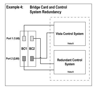
In these examples, the *dual* bridge cards are installed *in slots 9 and 10, so the maximum numbers of DSP card is 8.*
