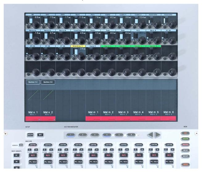
It is extremely easy to adjust a balance of e.g. a matrix output without accessing the fader strips of the contributing channels.
