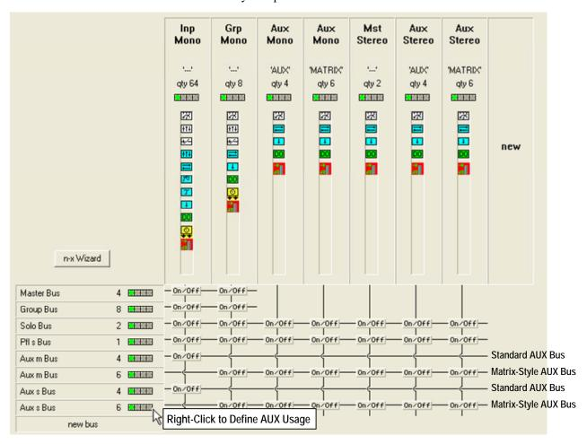
To avoid confusion about which master is a "true" auxiliary master and which one is a matrix output, it is recommended to rename the user label of the "matrix style" master channels to MATRIX 1, for example. This name will then be propagated and properly displayed on the input channels – as described at the beginning of these notes.
