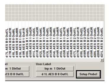
When clicking on this button the system brings up the set-up dialog and enters ProBel set-up mode.
