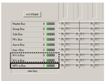
The required N–X m buses (dashed) and one MPX bus (solid) are added. If you use the N–X Wizard do not add the master Aux bus to mix the program to the MPX bus.
