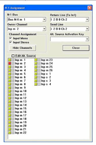
The new N–X bus type allows defining an "alternate N–X bus assignment". It is possible to select any console channel (or multiples) to be the alternate N–X output signal. This signal is activated by the ALT n–1 key on the channel strip. This can be done only if the owner channel's fader is closed.
