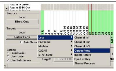
'Set Outputs' activates all preselected patch points to outputs on remote systems. This introduces an additional step in creating a patch connection, which the Vista SW did not know up to now.
