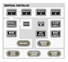
These keys have the same functionality as the ones on Vista 6 and 7. They allow fast access to the most important pages of the graphic controller screen.
