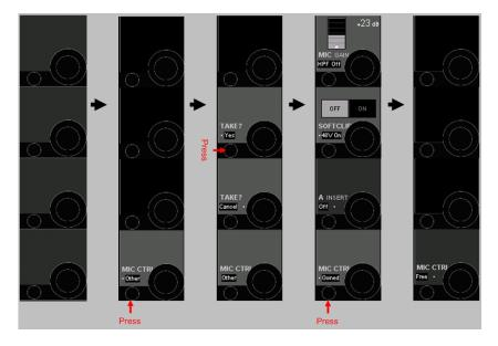
**1b** First, no mic is connected to the channel. Then, a shared mic currently *not* in use by another OnAir or Vista console is patched to the input channel manually:
