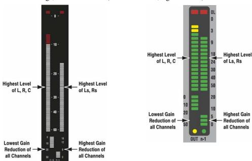
Discrete levels of all surround input legs are displayed in the *pan-ning window* of the Vistonics screen:
