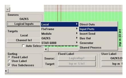
Shared inputs can be selected directly from any of the displayed systems. The sources of OnAir consoles – e.g. a DJ microphone – are appearing as 'Logical Inputs', and their output signals as 'Master Outputs'.
