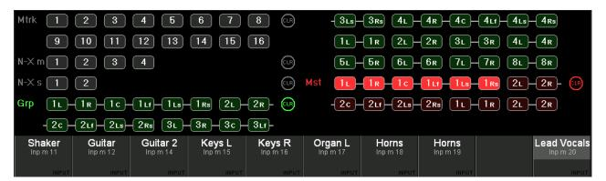
Only buses are shown here to which the current channel can be assigned. Pressing VIEW: BUS ASN on a master channel, however, will activate the "inverse bus interrogation" view described below.
