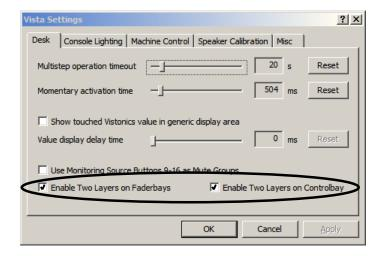
By activating "Enable Two Layers..." in the "Option: Vista Settings" menu, the virtual desk may be reduced from six to three sections. Scrolling will then be possible only between sections 1 and 3. The previous sections 4...6 now serve as a lower second (lower) layer of the console.
