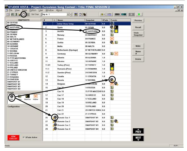
To create a cue, simply drag-and-drop one of the available **SNAPSHOTS** from the top left corner, or one of the **Events** from below the snapshots to the cue area. A cue can be created using the **Make** button on the right side of the cue list. It doesn't have to contain a snapshot; it is also possible to just fill in any event without activating any console setting changes.
