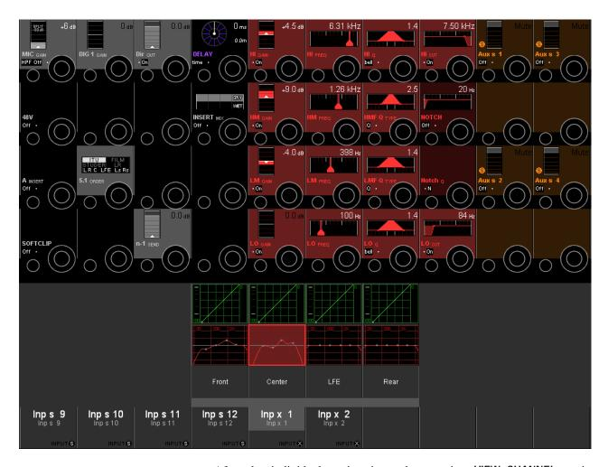
After the individual setting is made, pressing VIEW: CHANNEL again switches back to the standard channel view. In our case (where the front and center channels of Inp x 1 have individual EQ settings), the EQ field then displays the standard EQ curve with supplementary, small L, R and C characters, indicating that the front and center EQ settings are different from the displayed curve.
