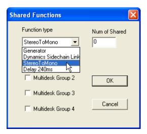
Note: It is also possible to configure one or multiple delays as a "shared process". However, in order to adjust its value you would have to be a system administrator and go into the "VMC tree" view of the console parameters. Hence this function is only intended when installing a console. Fixed delays might be set by Studer Service personal at that time.
