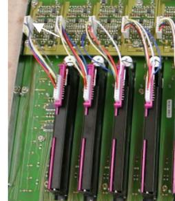
4. Remove the connector at the fader driver board
