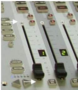
5. Remove fader knob the 2 attachment screws. The fader is now ready to be replaced
