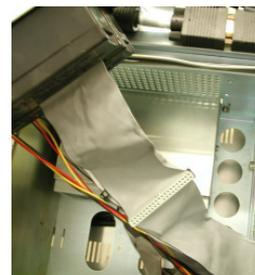
2. Disconnect IDE cables at mother-board and supply cable at distribution board. Carefully take cables back and remove frame with disk enclosures.
