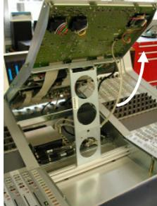
2. Swing the bay up into service position and lock it with the support leg.
