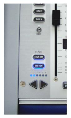
As long as the user wants to switch to a specific section, there is no difference in operation to the "layer" concept. Changing to another section is accomplished by pressing one of the corresponding keys in the **SECTION NAVIGATOR** area of the control bay, or by pressing the arrow keys located in each bay with **SCROLL: SECTION** set to ON (see left).
