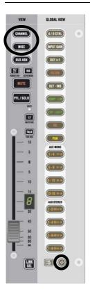
If the  $\Omega$  (shift) key is activated on a fader bay, it is possible to see up to 40 mono and 20 stereo auxiliaries when pressing MISC and CHANNEL on a channel strip. This is useful when working with multiple auxiliary and matrix buses.
