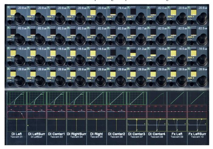
The touch screen area is also used for indication and operation of bus assignment:
