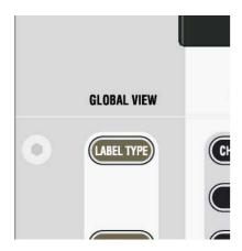
If the second layer option is activated, Vista 8 may display the label and real time metering of both layers at the same time. In order to activate this label view, press LABEL TYPE several times until the label display area on the Vistonics® screen shows the labels of both layers. This label of the second layer appears only if there is a channel assigned to that strip on both layers. Use the Strip Setup dialog on the graphic controller screen to do this.
