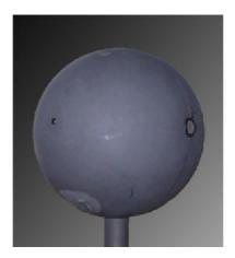
The Sphere setting is based on a microphone as shown in the picture above. Amplitude, phase and frequency response is calculated based on measured signals from such a microphone.
