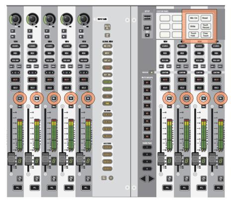
**Note:** The channel **ISO** keys are used for the 'Auto Mode' function in dynamic automation mode.
