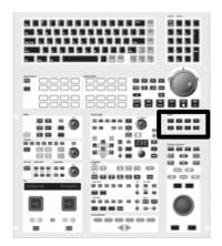
This area contains spare keys (F1...F3, F5...F7) for future functions and/or options. F4 is used for opening/closing the Clipboard Library window, F8 is used to activate external VGA input that allows to display an external VGA signal on the GC's TFT screen.
