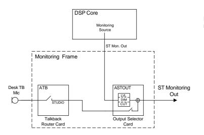
Features and drawbacks of analog talkback routing :
