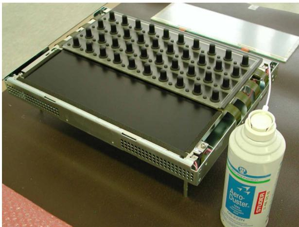
Clean the surface from dust, remove the protection foils from the new touch panel, insert the flexprints first (1) and place the new panel in its final position. It should firmly sit on the lower end (2) and be centered against the TFT.
