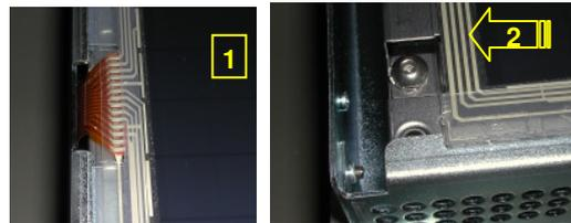
Verify that there is no dust between touch panel and TFT surface. Clean carefully with compressed air if required.
