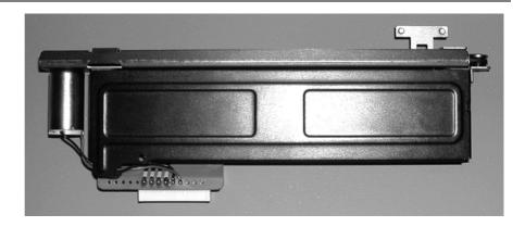
This paper describes how to service the Alps faders 1.950.044. Servicing is limited to cleaning the track substrate and slider assembly, and to lubricating the slider bearings.
