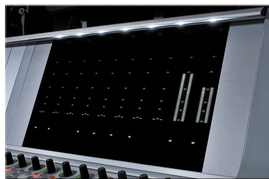
Optional illumination bar above the meter bridge, especially useful in dark environments like OB-vans or live applications.
