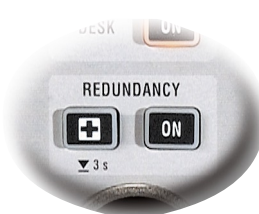
Redundant Control System switch.
