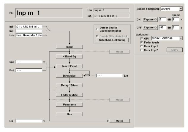
It is possible to control faders of all console channels externally. When using this feature, the console operator determines the "Fader Open/Close" values, as well as the speed the fade in/out should happen. Various triggers are available in order to activate the fade. The channel patch window allows adjustment of all necessary settings.
