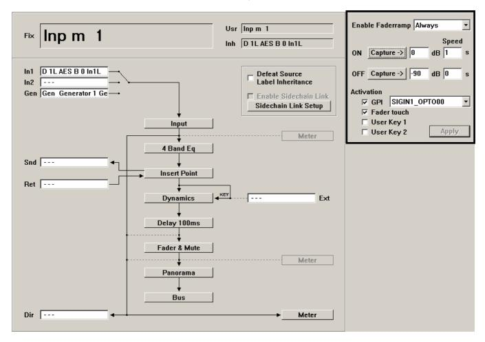
Faders of all console channels can be externally controlled. When using this feature, the console operator determines the Fader Open/Close values, as well as the fade in/out speed. Various triggers are available in order to activate the fade. The channel patch window allows adjustment of all necessary settings.
