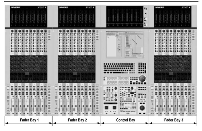
The desk consists of two types of bays: *Up to seven* identical fader bays and *exactly one* control bay.
