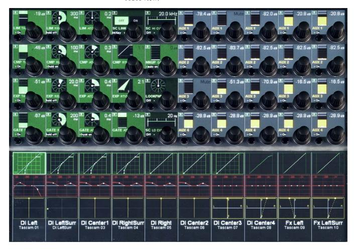
This philosophy is completed by three hardware keys underneath the Vistonics<sup>TM</sup> display, showing different combinations of parameters as well as the bus assignment of that specific channel, covering the whole Vistonics<sup>TM</sup> area.
