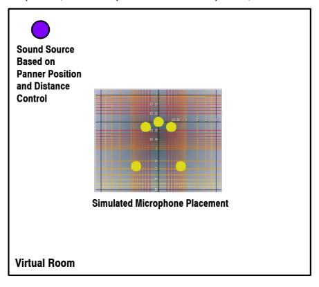
The dry signal within a VSP channel is now placed to an imaginary position based on the panner positioning within the channel. You can now imagine that, if each speaker (in your monitoring environment) is fed the signal based on the placement of the "microphones" in the simulation (including the reflections), that a realistic sound space could be achieved. This is a simplification of what happens within the VSP system.
