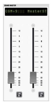
Vista 8's control bay also hosts two "grand master" faders. The user determines which two faders are most important for him and to which he wants constant access. This may be very useful as an "emergency access" to very important output faders, since these faders will never scroll or be switched over in any way. Which two channels are controlled by these faders is defined in the top right corner of page 2 (Control Bay tab) of the strip setup window, as shown below.
