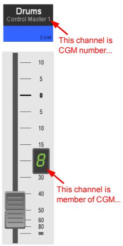
D950: On the D950 it is not possible to see, to which CGM a CGM may belong. A small light next to the fader shows the presence of another hierarchical level.
