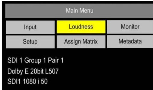
The **Loudness Setup** menu may be used to define the parameters used to measure **Loudness** using the **ITU-R BS1770** algorithm, to select and set the specific audio channels under test and to start/stop measurement manually. The resultant **Loudness** measurement may be observed via either the **Bargraph Display** or from the **Loudness Histogram** which is accessed via the **Data** button.
