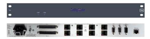
The TallyMan controller should be installed in a standard 19" rack with good ventilation, no other special precautions need be taken, further information regarding earthing, mounting, power etc may be found in the **Safety** section.
