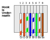
For a hub connection, use a straight-through cable. For TallyMan Controller to Computer, use a crossover cable
