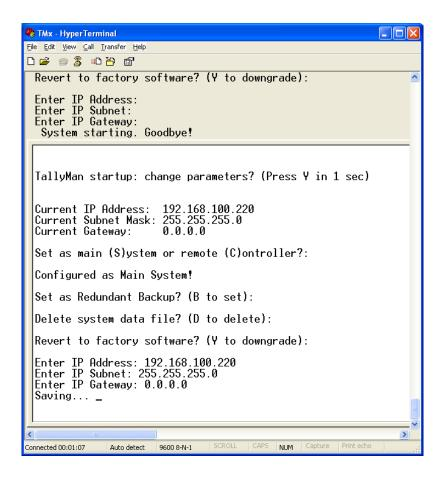
Start HyperTerminal and then power up the TM1 and wait for about 10 seconds. Press Y on the keyboard within 1 sec of the message appearing. Follow the on-screen instruction
