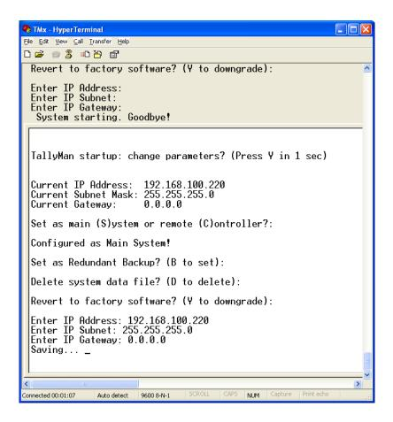
Start HyperTerminal and then power up the TM2+ and wait for about 10 secs. Press Y on the keyboard within 1 sec of the message appearing. Follow the on-screen instruction
