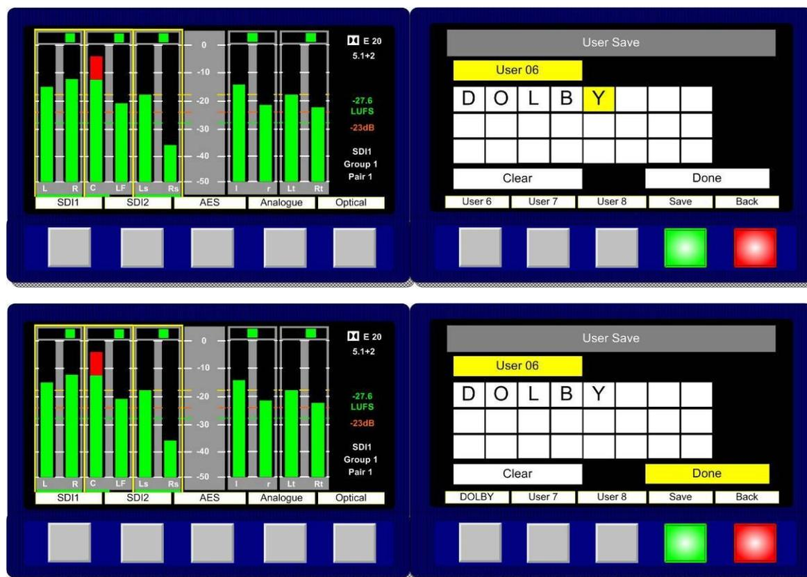
To recall a **User Preset** which isn't stored on **Preset Recall** buttons 1-8, rotate the **Encoder** clockwise to activate the **User Preset** window in the right hand OLED screen. Highlight and select to recall a **User Preset** from locations **U01** to **U24**.
