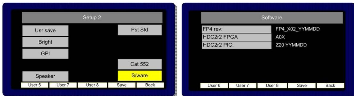
Press button 10 to exit the **S/Ware** mode and insert the SD card. Then re-enter **S/Ware** mode, a new menu option should have appeared at the bottom of the screen. Highlight and select **Perform Update**.
