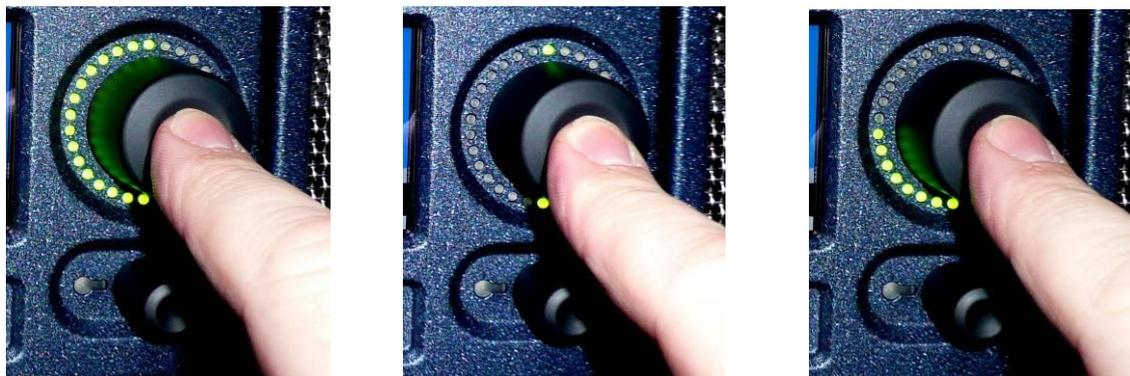
The **Setup 2 Menu** contains a button to select the operational brightness of the switch and encoder LEDs. By selecting and rotating the encoder the overall brightness of the LEDs may be changed from low to high level across 5 graduations. 1 is low, 5 is high.
