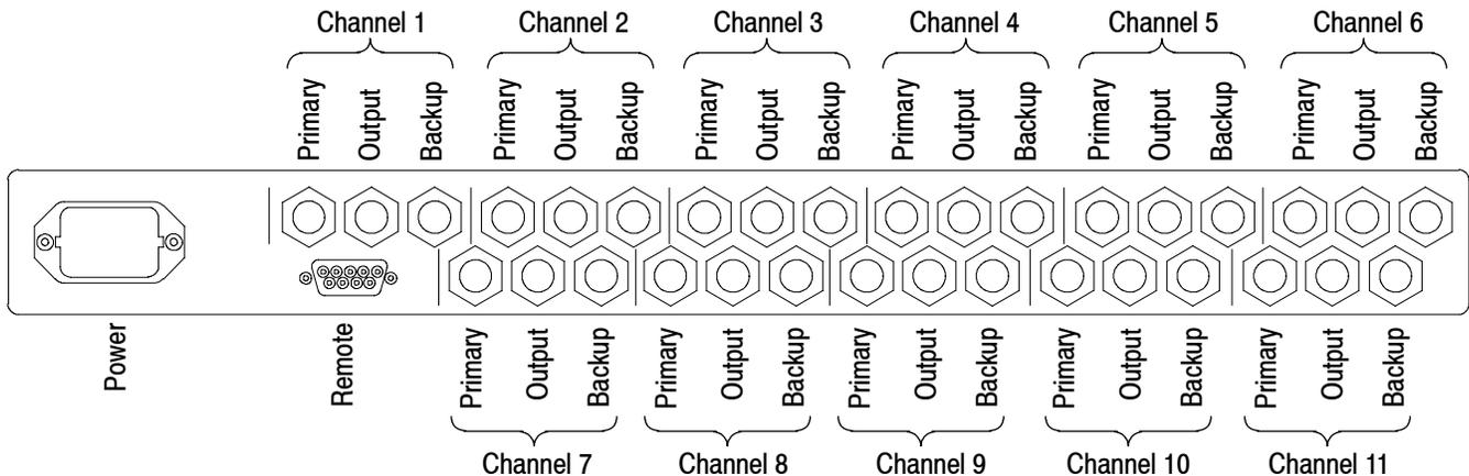
Figure 1-3: Rear panel of the ECO422D
