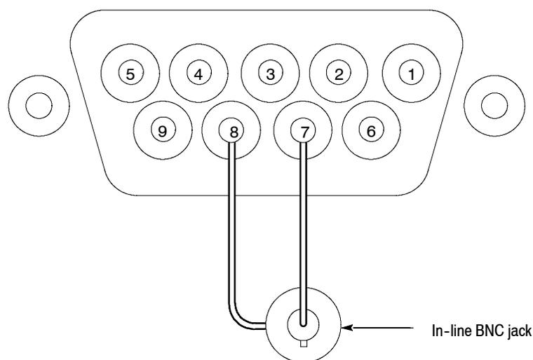
**Figure 1-5: Wiring required to conform with SMPTE fault reporting**
