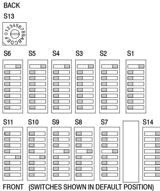
**Figure 1-2: Default position of the user configuration and mode switches**
