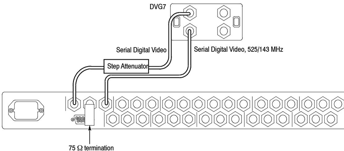
**Figure 4-3: Setup to check the serial digital video composite levels**
