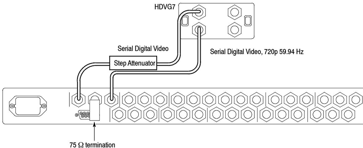
**Figure 4-5: Setup to check the component serial digital video levels**
