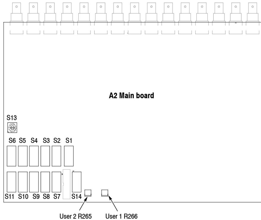
**Figure 1-7: Selection switches and user level control locations**
