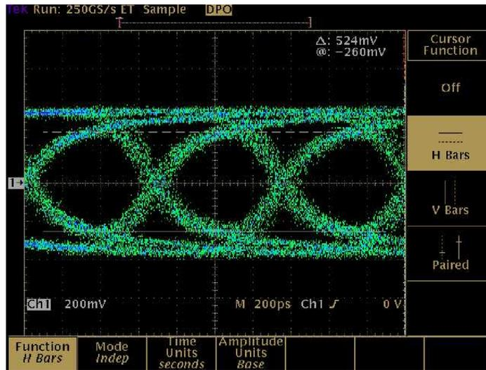
Figure 2-1: Typical eye-pattern of 20 m of Belden 1694A cable
