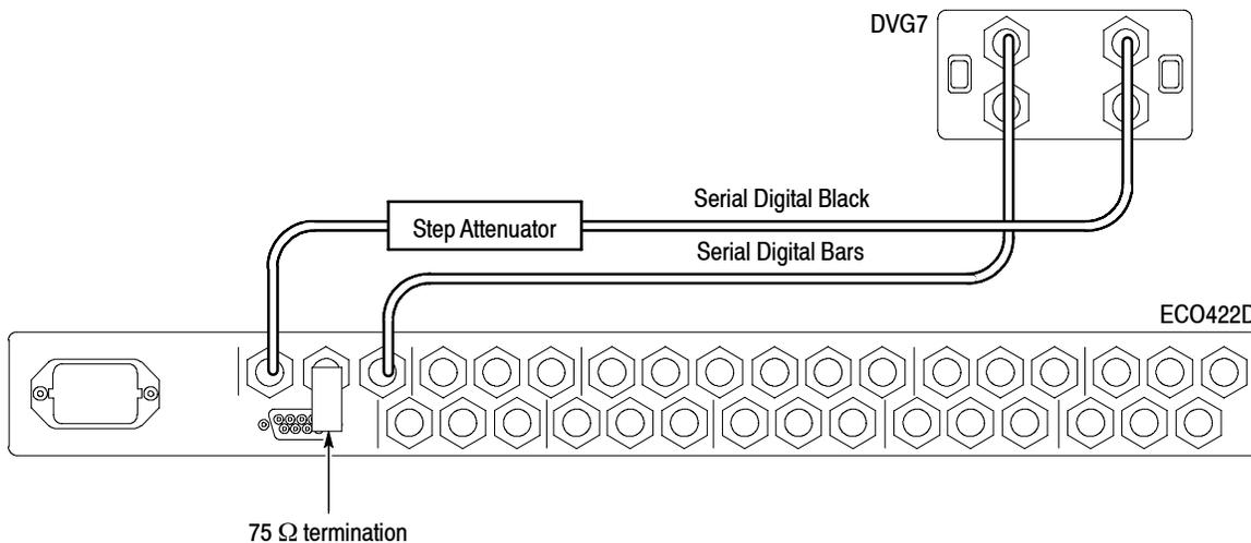
**Figure 4-2: Setup to check the component serial digital video levels**
