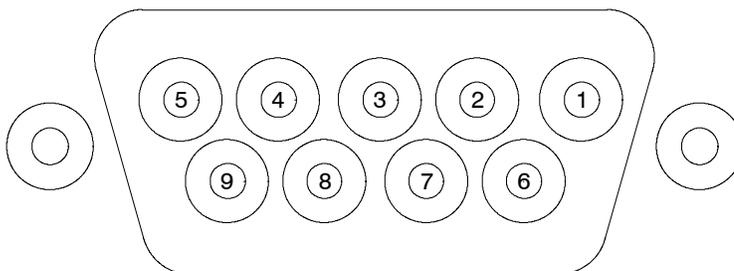
**Figure 1-4: Remote connector pins**
