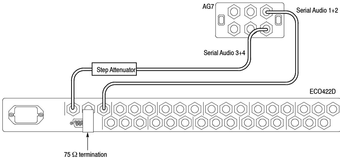
**Figure 4-4: Setup to check the serial audio levels**
