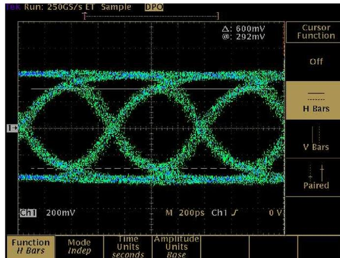
Figure 2-2: Typical eye-pattern of Channels 1-6 HD output (Channels 1-3 with Opt. ELSW)
