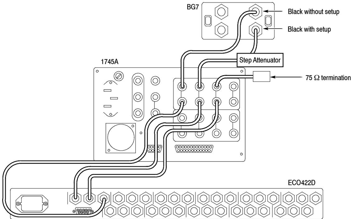
**Figure 4-1: Setup to check Black Burst levels**
