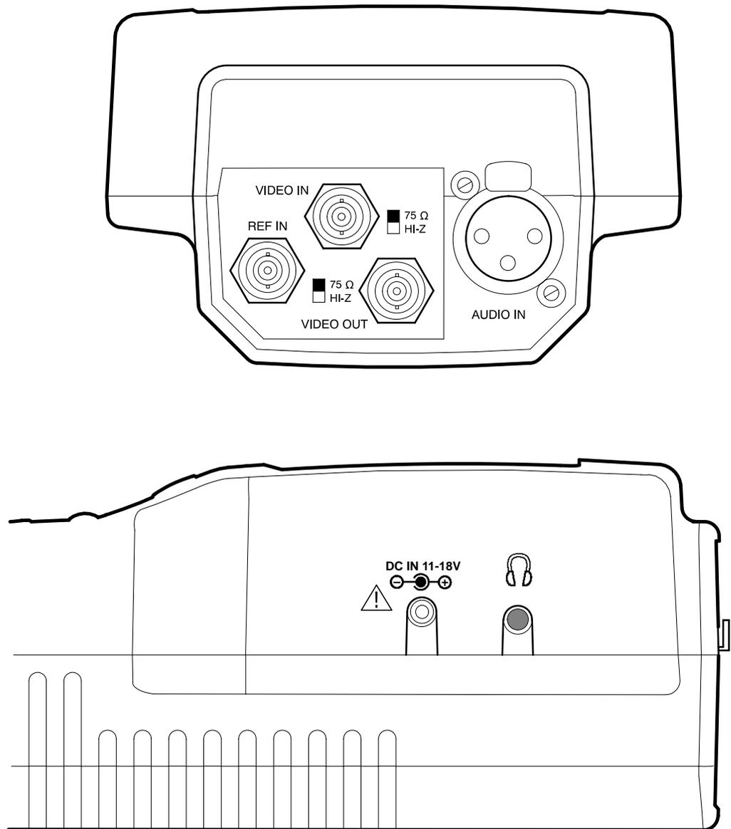
Figure 2-2: WFM 90 and WFM 91 side panels
