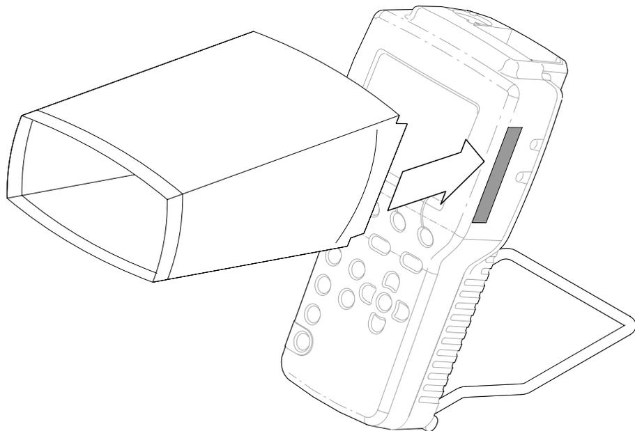
Figure 1-4: Installing the viewing hood
