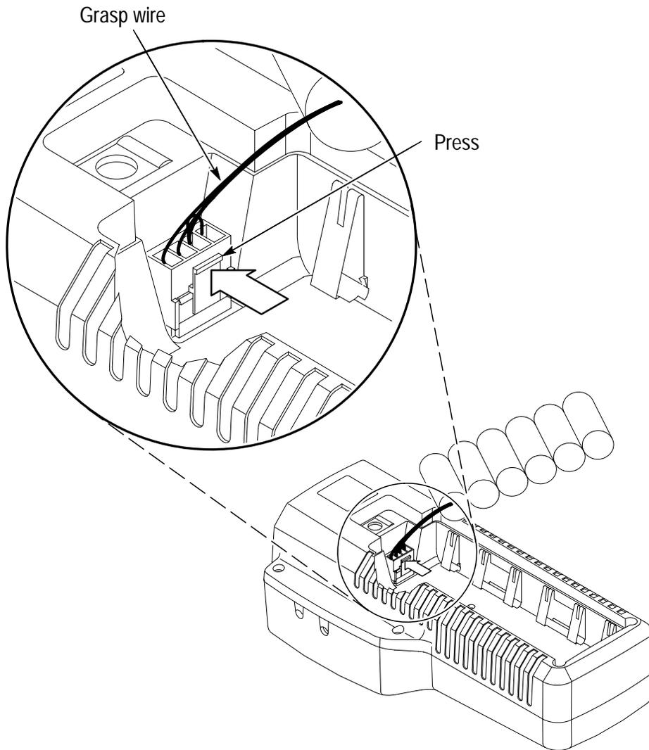
**Figure 1-3: Removing the NiCad battery pack**
