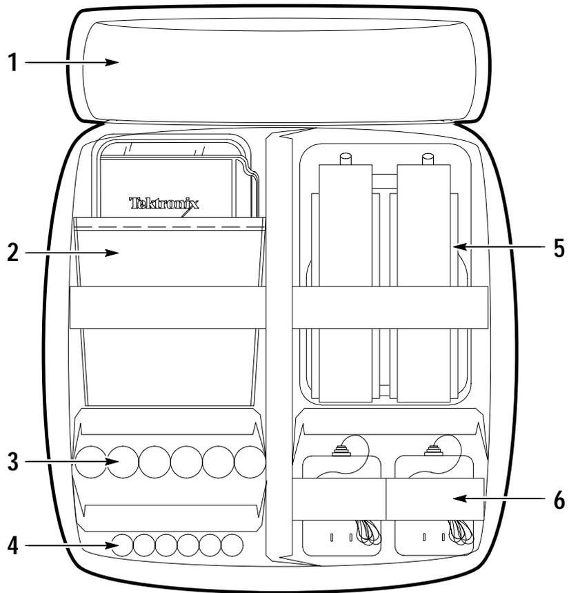
**Figure 1-1: Packing the Option 33 travel case**
