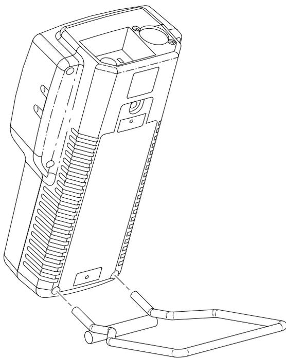
**Figure 1-5: Installing the desk stand**
