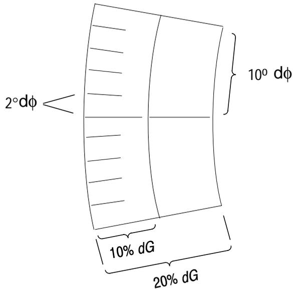
Figure 3-6: Differential gain and phase measurement box
