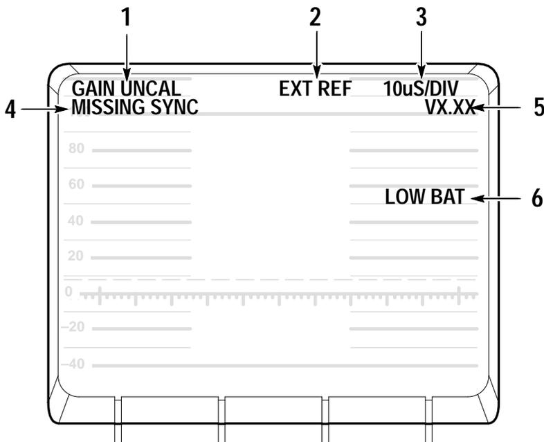
**Figure 2–3: On-screen readout messages**
