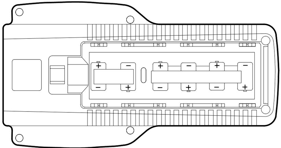
**Figure 1–2: Installed polarity of alkaline batteries**
