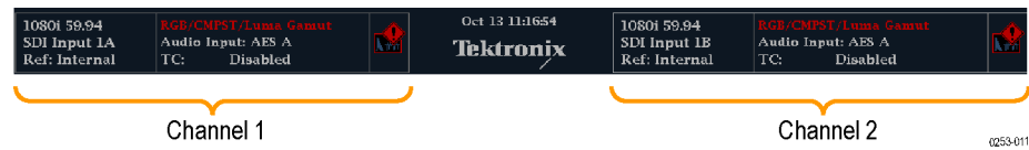
Figure 8: Status bar in simultaneous input mode
