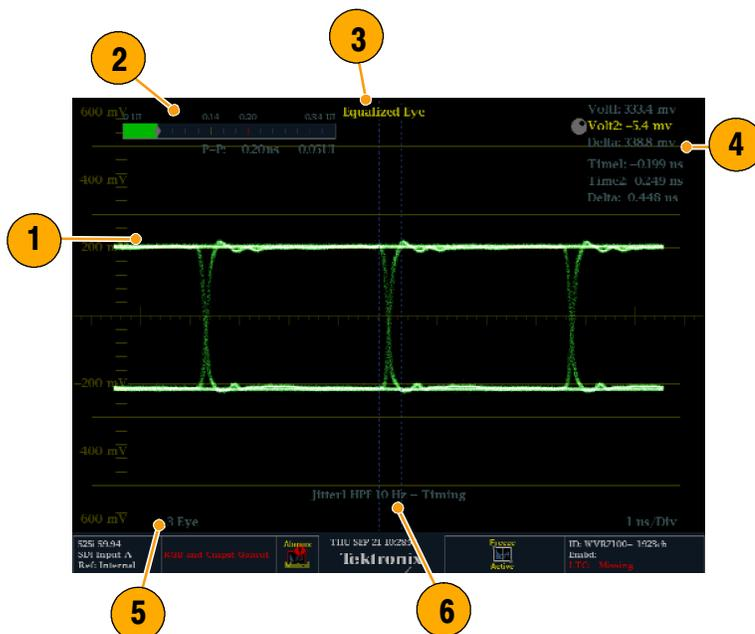
At the end of a long cable, the eye diagram may appear so noisy that there is little or no discernable opening. In this situation, limited use of the eye diagram is still possible by selecting Equalized Eye mode. The equalizer compensates for the effects of cable length by applying an inverse response function and then reslicing the signal to a logic level. This causes amplitude information to be lost, but preserves the effects of jitter in the signal.
