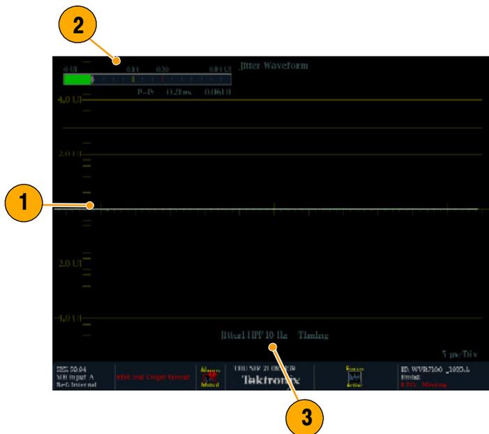
**High-Pass Filter.** The high-pass filter bandwidth setting allows you to show only jitter terms above the selected filter frequency. When you select a filter setting, depending on the active input signal, you select the jitter measurement type (Timing, Alignment, or neither, as defined by the SMPTE standard). Use the High Pass Filter soft key to select the lowest settings to measure timing jitter and the higher settings to measure alignment jitter.
