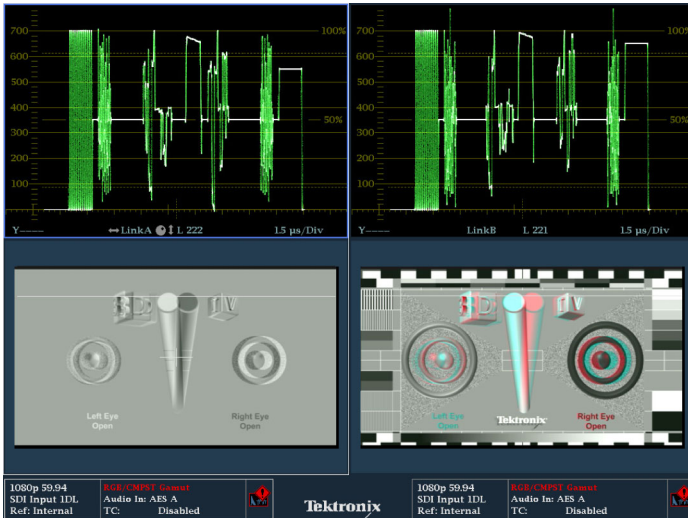
3D Left and Right Eye images showing a Difference Map and Red/Cyan Anaglyph using SIM mode.
