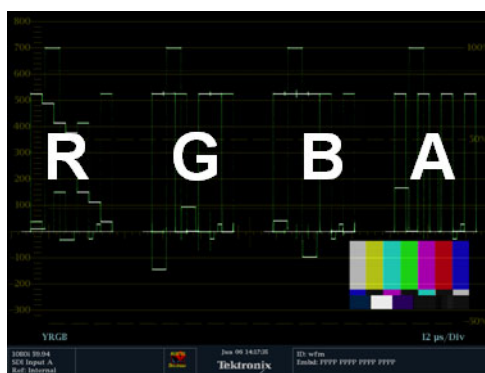
Figure 14: Dual Link information placement in waveform display
