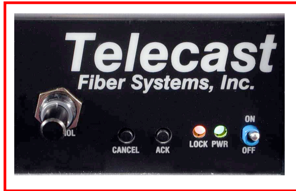
Figure 16: Local gain controller/selector
