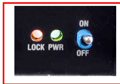
Figure 6: Link LOCK Status LEDs
