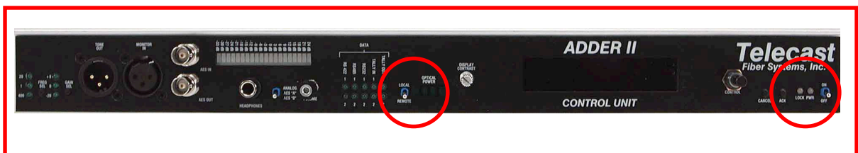
Figure 4: Optical Power Display and LINK LED Location, Front panel
