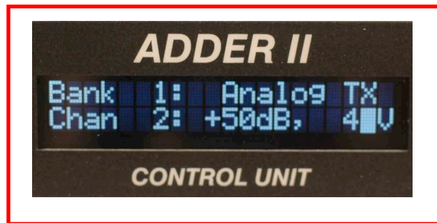
Figure 21: Setting Phantom Voltage
