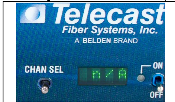
Figure 5 : n/a indicates no optical link
