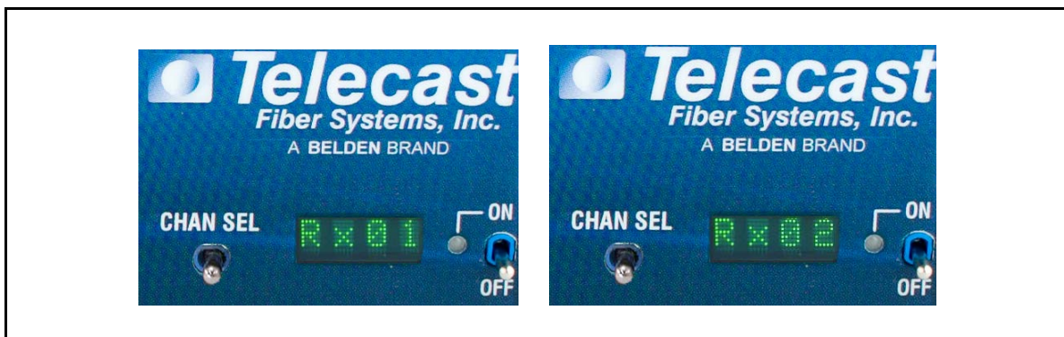
Figure 4: using the toggle to change channels to be monitored
