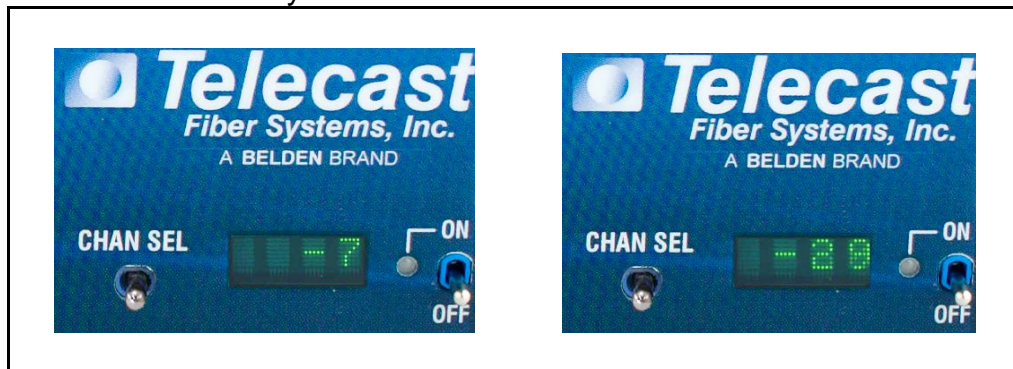
Figure 6 : Variable optical power levels = NO SDI present
