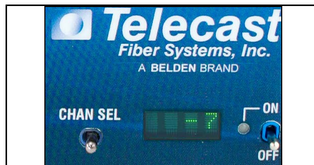
Figure 7: A steady numerical value IS the received optical power for that channel.
