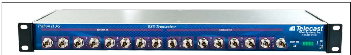
Figure 3: Front Panel, 8 Channel bidirectional CWDM Transceiver
