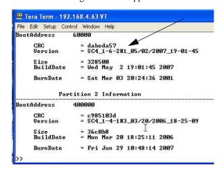
The version (pointed to above) is the device's current software version, for the indicated device - in this case an SC-4.
