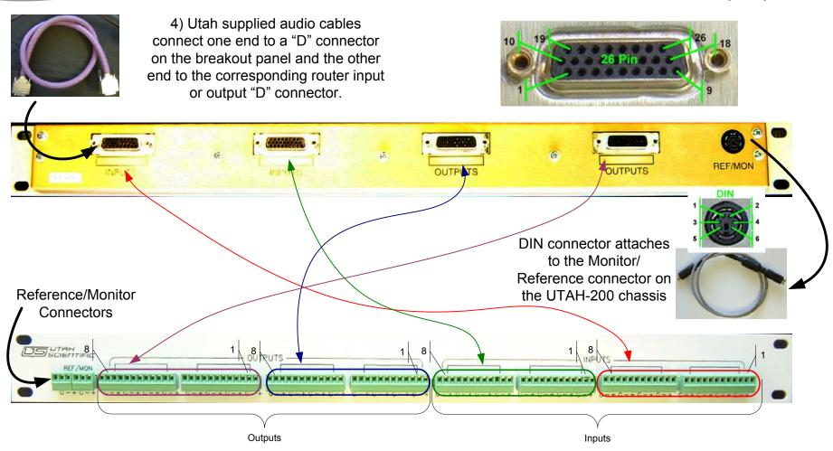
Note: each "D" connector/terminal block set provides connections for router eight inputs or outputs.
