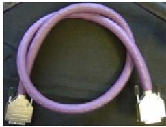
4) Utah supplied audio cables connect one end to a "D" connector on the breakout panel and the other end to the corresponding router input or output "D" connector.
