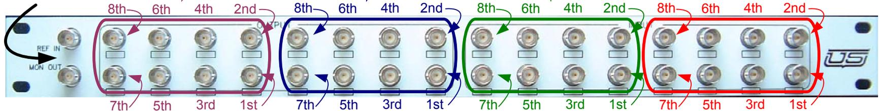
Note: The numbering on each set of eight BNC's indicate which input or output the BNC is connected too. For example: If the far right (red) set of eight were connected to the "D" connector on the router for inputs 00 to 07, the BNC labeled "1<sup>st</sup>" would be connected to Input 00, "2<sup>nd</sup>" would be input 01 and so forth.
