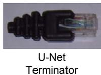
U-Net connectors connect to a U-Net port on the SC-4/400 or to a loop-through from another panel via a typical CAT-5 cable. U-Net must be terminated at the end of the loop-through with the supplied U-Net terminators. Maximum cable length of 1000 feet per run.
